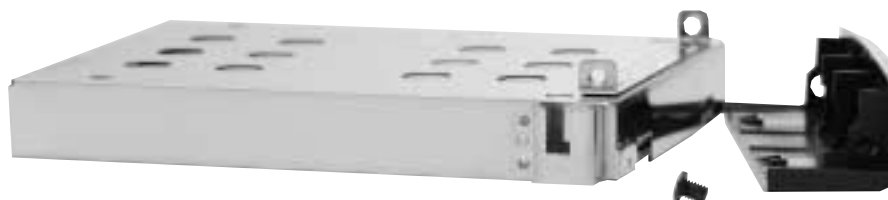
Figure 8.8: Removing the Bracket from the Hard Disk Drive
