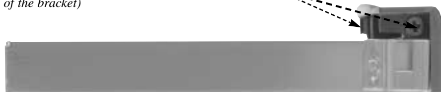
Figure 8.7: Removing the Bracket Screws (both ends of the bracket)
