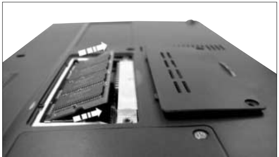
Figure 10.2: Replacing the Memory Card
