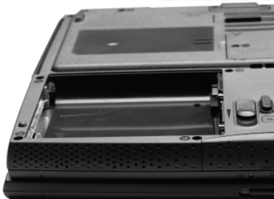
Figure 4.2: Changing the Battery
