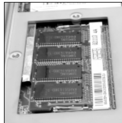
Figure 4.3: Replacing the Memory Card
