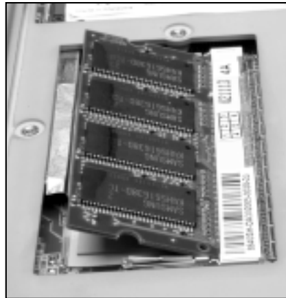
Figure 4.2: Replacing or installing RAM
