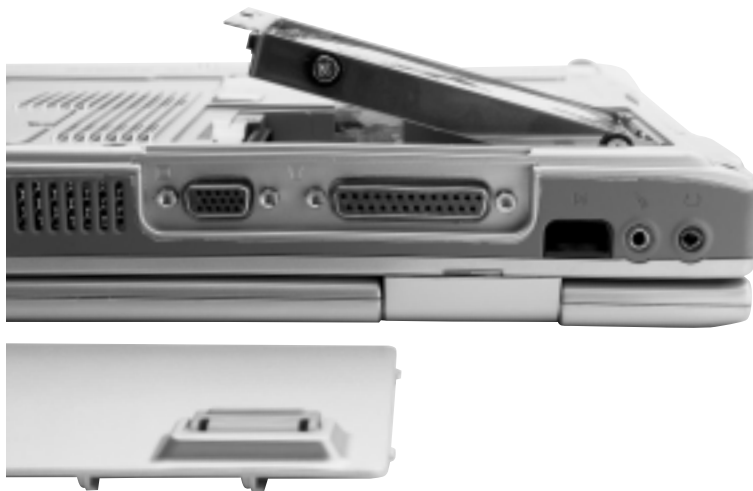
Figure 10.6: Replacing the Hard Disk Drive
