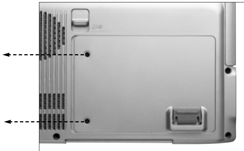
Figure 10.5: Removing the Hard Disk Drive Screws
