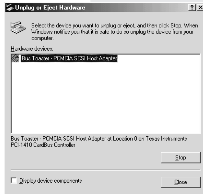
Figure 5.5: Ejecting a PCMCIA Card
