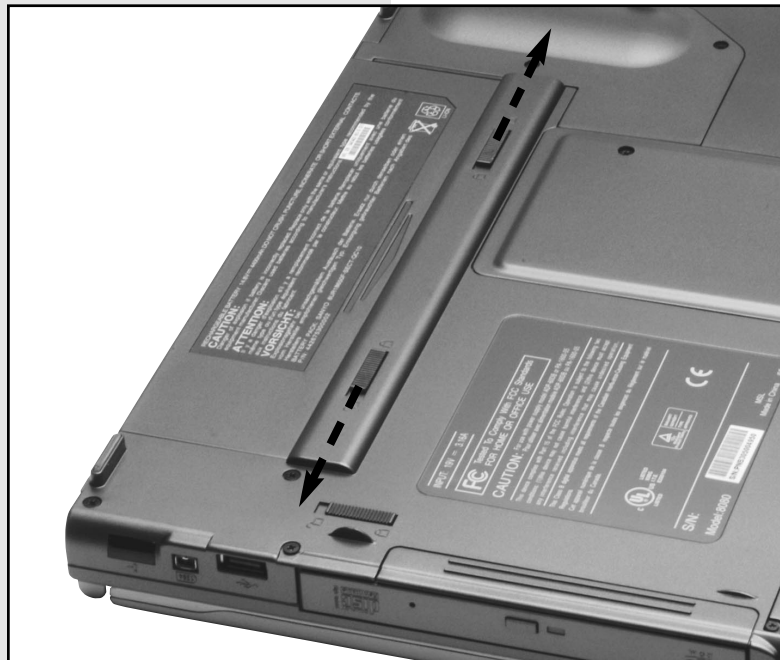
Figure 3.2: Changing the Battery
