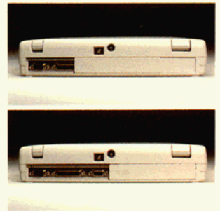
A sliding door is built into the computer case to protect interfaces.
