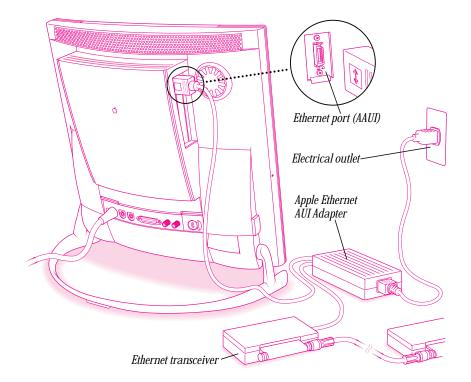
**5** Plug the connector on the Apple Ethernet AUI Adapter into the AAUI Ethernet port on your computer.
