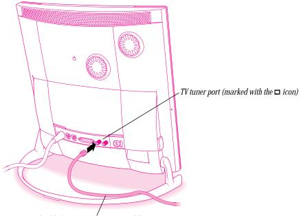
Coaxial cable from a TV antenna or cable TV service
