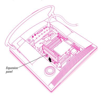
5 Plug the communication card adapter into the computer's communication card expansion slot.
