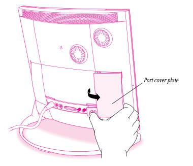
2 Set the cover plate aside. (The cover plate is made up of two sections that can be easily separated and reassembled if needed.)
