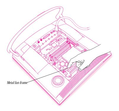
**3** If your computer has a communication card, remove it and the expansion panel as shown in the illustration.
