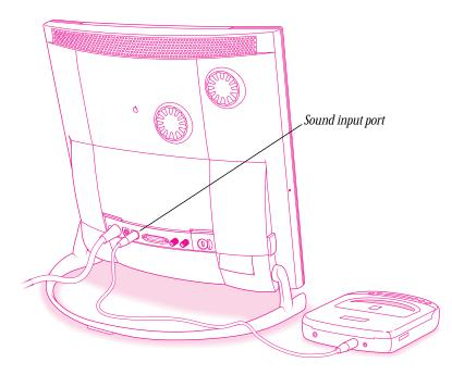
**5** If your audio equipment is a sound output device such as headphones or amplified speakers, attach its cables to one of the sound output ports.
