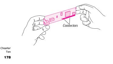
**7** Align the end of the communication card with the expansion panel.
