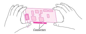
**5** Attach the PCI card adapter to the PCI card.
