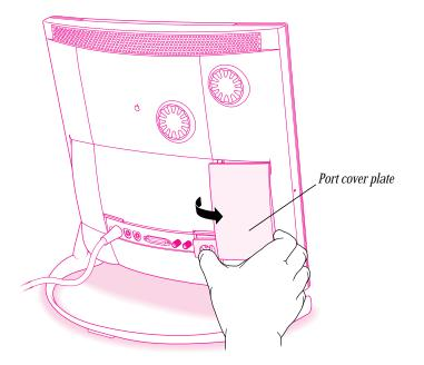
The port cover plate covers the ports for connecting a modem, keyboard, printer, and video equipment (such as a video cassette recorder or camcorder).
