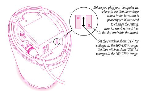
2 Plug the socket end of the power cord firmly into the recessed power plug (marked with the symbol ∼) inside the well on the bottom of the bass unit.
