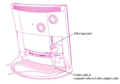
**Important** The S-video connector is a round plug with several small metal pins, which resembles other Macintosh connectors, such as those for a printer, modem, mouse, or keyboard. Don't confuse the connectors; they're not interchangeable.
