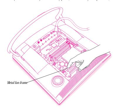
2 If you need to remove one or more existing DIMMs to make room for new ones, remove them now. Hold the DIMM along its side edges, and press down on the ejector as shown. The DIMM will be released from its slot. Pull the DIMM straight up and out of the slot.
