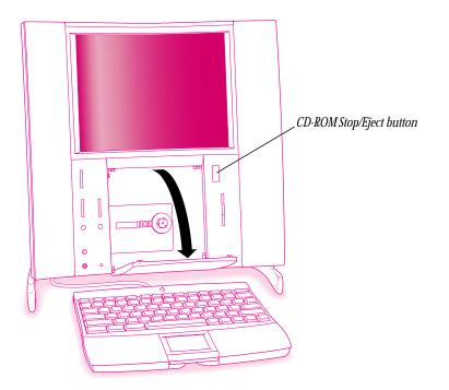
**2** Press the center of the disc onto the CD-ROM drive's spindle, label side out.
