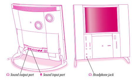
You need a cable with one of the 3.5-mm audio connectors shown below to connect equipment to your computer's sound input port. You need a cable with a stereo miniplug to connect speakers or other equipment to the sound output port.
