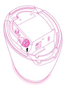
4 Plug the connector at the end of the computer's cable into the bass unit's connector.
