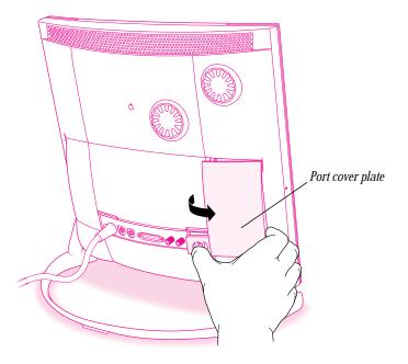
3 Attach the LocalTalk adapter to the printer port (marked with the 🗉 icon) located behind the cover plate you removed, and press the cable into the cable guides. Then attach a network cable between the LocalTalk adapter connected to your computer and the last LocalTalk adapter on your existing network.
