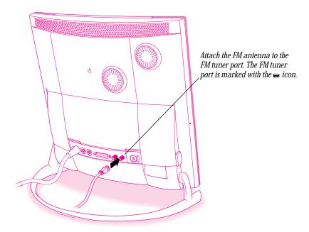
Chapter Seven **3** Unfold the FM antenna and position it high for the best reception.
