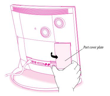
The port cover plate covers the ports for the modem (or GeoPort Telecom Adapter), keyboard, printer, and video equipment.
