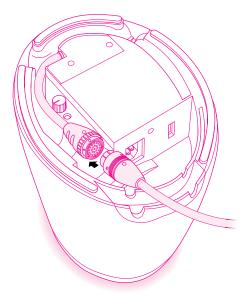
Chapter One **10**  **5** Secure the connection by very firmly rotating the metal band until you hear a click.
