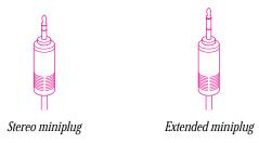
The stereo miniplug is the smaller of the two and is found most often on stereo equipment. The extended miniplug, which is slightly longer and comes with voice quality external microphones (such as the Apple PlainTalk Microphone), works only in your computer's sound input port ( $\Psi$ ).
