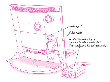
**2** Plug one end of the adapter's telephone cord into a telephone jack. Plug the other end into the line port on the adapter.
