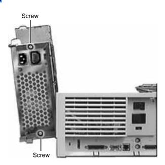
4 From the back of the computer, remove the two screws that secure the power supply to the chassis.
