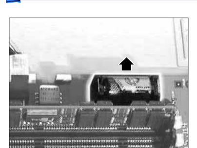
2 Lift up the battery to remove it from the logic board.
