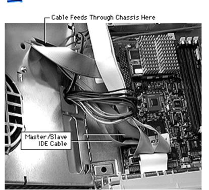
The graphic at left shows how the split master/slave IDE cable connects to the logic board. The same connector is used for both the regular IDE cable and the master/slave IDE cable that connect to the CD-ROM and Zip drives, depending on which one comes with the unit.
