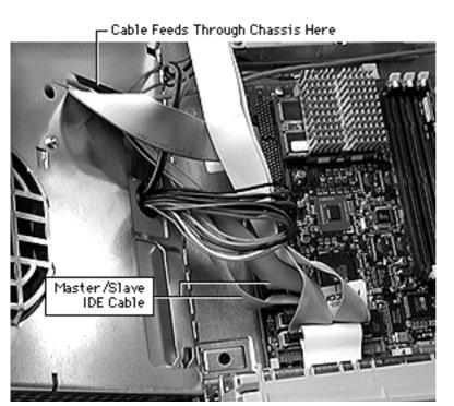
The graphic at left shows how the split master/slave IDE cable connects to the logic board. The same connector is used for both the regular IDE and the master/slave IDE cables.
