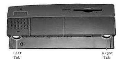
Press the two tabs at the front corners of the top housing to release the top housing from the bottom chassis.
