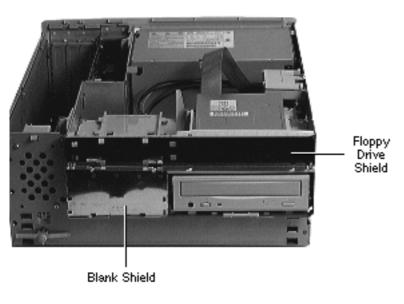
Remove the blank shield and the floppy drive shield from the front of the unit.
