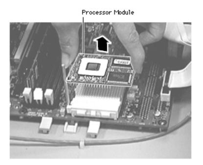
6 Pick up the processor module by the edges and gently lift straight up to remove it. Be careful not to bend the pins underneath the module.
