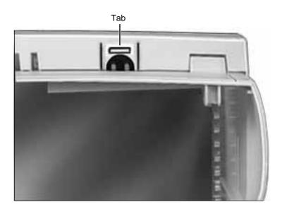
1 From the underside of the top housing, pull out on the moon-shaped opening at the bottom of the bezel to release the tab. Lift up the bezel to remove it from the top housing.
