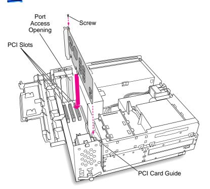
4 Align the card connector with the expansion slot and press straight down until the connector inserts all the way into the slot.
