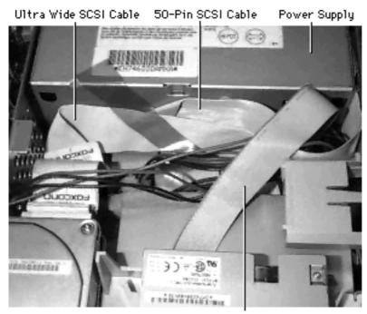
Route the ultra wide SCSI cable on top of the 50-pin SCSI cable and tape them both to the power supply. The ultra wide SCSI cable must be away from the CD-ROM drive, and the floppy cable should be routed on top of the other cables.
