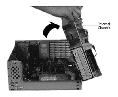
Swing open the internal chassis that contains the power supply. Be sure the internal chassis is perpendicular to the bottom chassis and fully supported by the chassis support foot.
