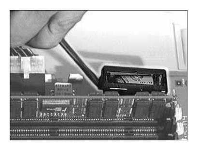
1 Use a screwdriver to gently pry up one side of the battery cover.
