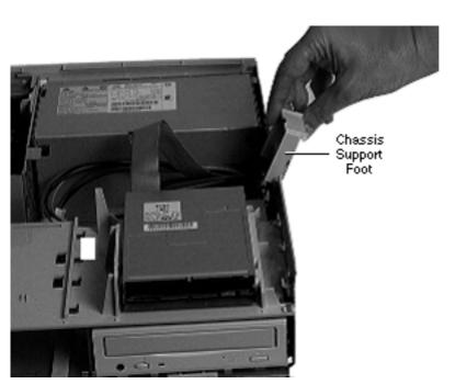
2 Flip out the chassis support foot.
