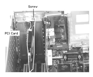
1 Remove the screw that secures the PCI card to the back of the chassis.
