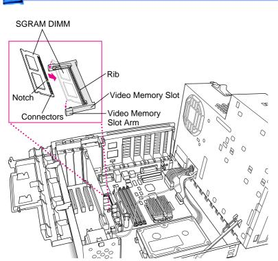
2 Align SGRAM DIMM notches with VRAM slot ribs.
