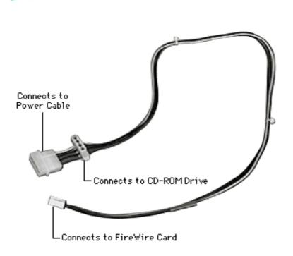
**Note:** The graphic at left shows the internal FireWire cable and each of its connectors.
