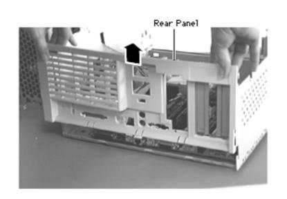
I Lift the rear panel straight up to unhook it from the metal chassis.
