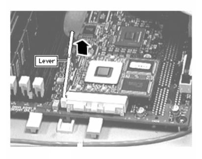
Lift the metal lever at the left of the processor module.
