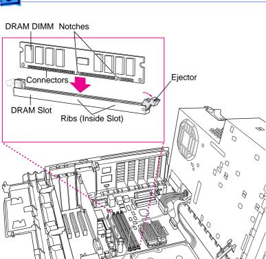
2 Align DIMM notches with DRAM slot ribs.
