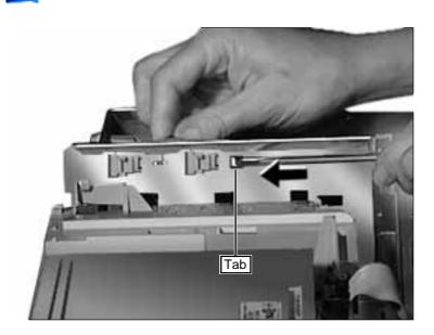
1 Use a screwdriver to push out the tab indicated in the illustration. Slide the latch forward and lift it from the chassis.
