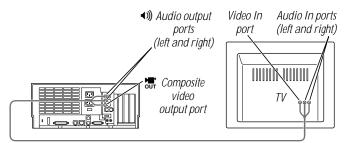
Triple RCA-plug cable (available at most electronics supply stores)
