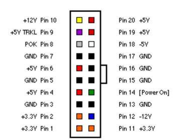
Figure 1. Power Supply 20-Pin Connector
