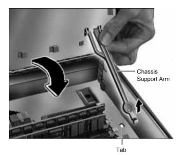
5 Release the chassis support arm and swing down the internal chassis.
