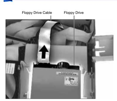
3 Disconnect the floppy drive cable from the back of the floppy drive.
