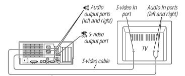
Dual RCA-plug cable (available at most electronics supply stores)
