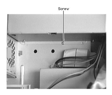
Remove the screw that secures the power supply to the bottom of the internal chassis
