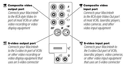
The S-video input and output ports accept S-video connectors, and the composite video input and output ports accept RCA-type connectors.
