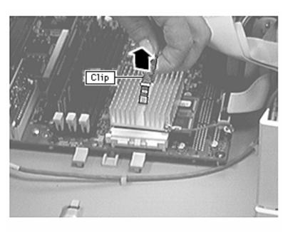
Lift up the clip and remove it from heatsink.
