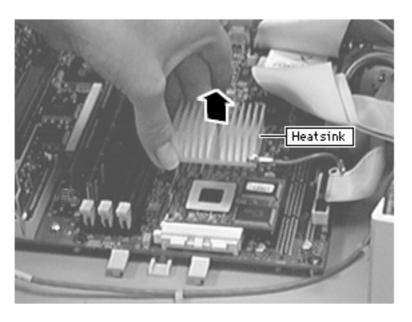
Lift up the heatsink to remove it from the processor module.
