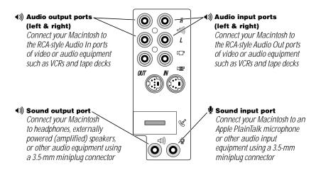
The left and right RCA-type ports accept this type of connector:
