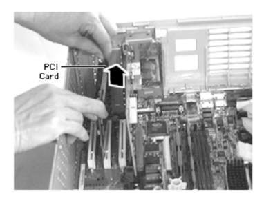
2 Grab the corners of the PCI card and pull up the card to remove it.
