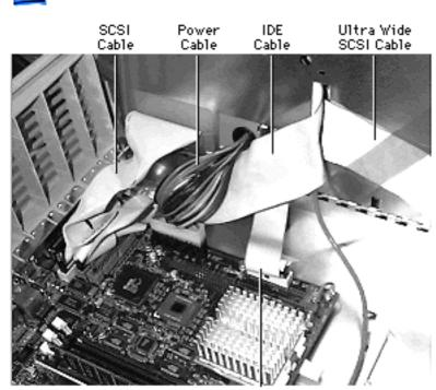
Feed the ultra wide SCSI cable through the first cut out in the drive chassis.
