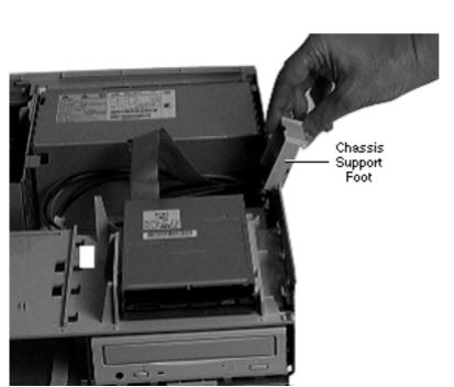
2 Flip open the chassis support foot.
