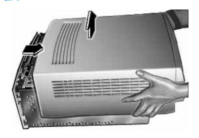
Pull the top housing forward about 1 to 2 inches and lift straight up to remove the top housing from the computer.
