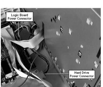
3 Disconnect the power supply cable from the hard drive and the logic board.
