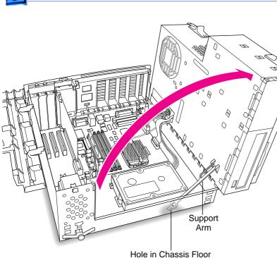
4 Swing the chassis up and insert the support arm in the hole.
