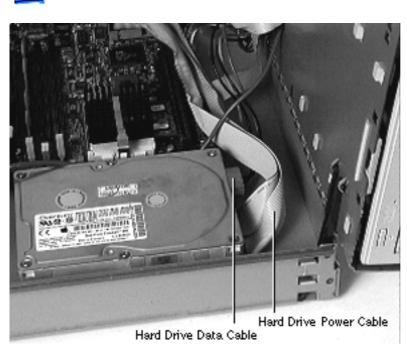
1 Disconnect the cables from the hard drive.
