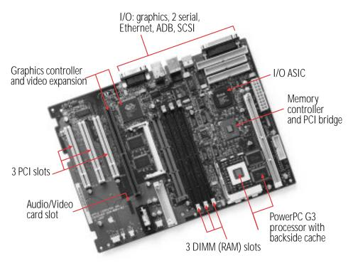
Memory. The memory controller and PCI bridge support the Power Macintosh G3 systems' three memory slots and three PCI expansion slots. These systems make use of a faster, industry-standard memory, SDRAM, which adds to both their economy and their availability.
