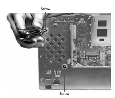
2 Remove the two Torx screws that secure the speaker to the metal chassis.
