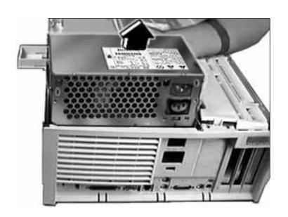
7 Slide the power supply forward and pull it out of the computer. You will need to feed the power supply cables that connect to the logic board up through the hole in the chassis.
