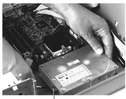
2 Pull up the release tab at the front of the hard drive and push the back of the hard drive to remove it from the drive chassis.
