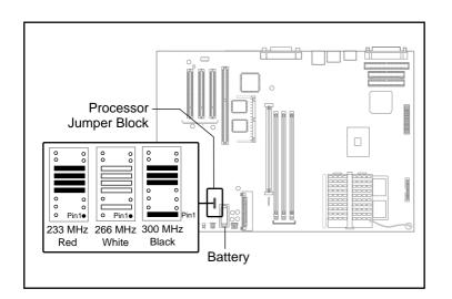
The graphic at left shows the proper installation for the processor module jumper. Depending on the computer's processor speed, you will either install a red jumper (233 MHz), a white jumper (266 MHz), or a black jumper (300 MHz). Be sure to cover the pins as shown and to install the jumper block with the gold connector pins facing down towards the board.
