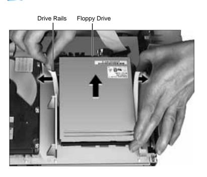
4 Pull out on the plastic drive rails that secure the floppy drive to the drive chassis and push back the drive to release it.
