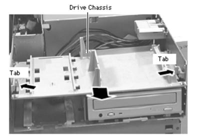
1 Push in on the two tabs securing the drive bracket to the internal chassis and slide the drive bracket out to remove it.
