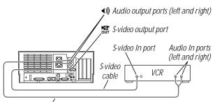
Dual RCA-plug cable (available at most electronics supply stores)
