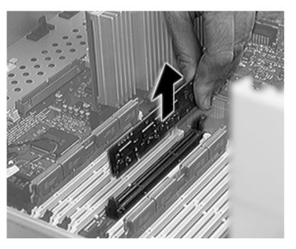
4 **Caution:** Hold the DIMM by the edges, not the chips.
