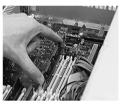
**Replacement Caution:** The DIMM is keyed so that it fits into the DIMM slot only one way. Be sure to align the notches in the DIMM with the small ribs inside the slot.
