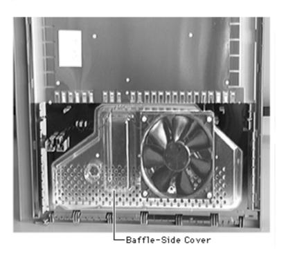
I The baffle has adhesive along its edges. Press the baffle into place as shown.
