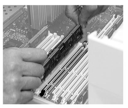
**Replacement Caution:** The DIMM is keyed so that it fits into the DIMM slot only one way. Be sure to align the notches in the DIMM with the small ribs inside the slot.
