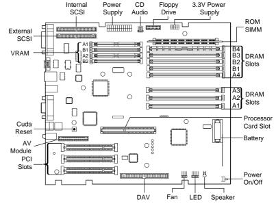
Figure: PM 8600/250 & 8600/300 Logic Board
