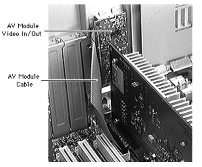
4 Disconect the AV module cable from the logic board.
