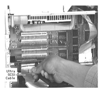
1 Grip the pull tab on the Ultra Wide SCSI cable and pull to disconnect the cable from the Ultra SCSI card.
