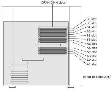
Figure: PM 9600/WS 9650 DRAM DIMM Slots
