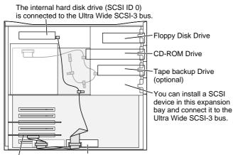
SCSI PCI Card One 5.25" Hard Disk Drive or two 3.5"Hard Disk Drives can be installed on the floor of the server and connected to the Ultra Wide SCSI-3 bus. (Some Workgroup Server models come with a second Hard Disk Drive [SCSI ID 1] installed here.) Replacement Note for WS
