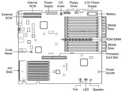
Figure: PM 9600/WS 9650 Logic Board
