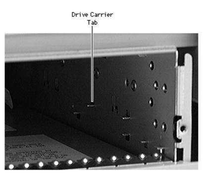
**Replacement Note:** When inserting the drive into the computer, make sure the drive carrier aligns with the carrier guides. The carrier should slide between five metal tabs below and two metal tabs above the left and right edges of the carrier.
