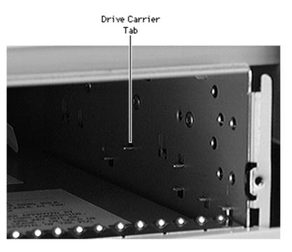
**Replacement Note:** When inserting the drive into the computer, make sure the drive carrier aligns with the carrier guides. The carrier should slide below the four metal tabs on the left and right sides of the drive bay.
