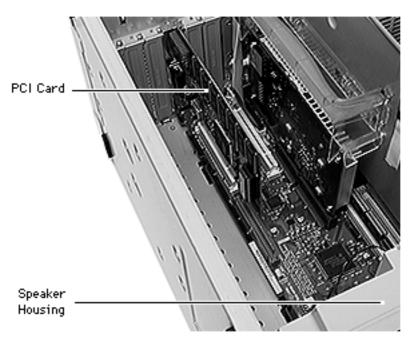
3 **Note:** For longer PCI cards, slide the end of the card opposite the connector into the appropriate slot in the speaker housing.
