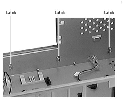
Using a flat-blade screwdriver, release the six latches holding the stationary panel to the chassis.
