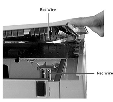
**Replacement Caution:** Make sure the red fan cable wire in the speaker housing matches up with the red fan cable wire in the side access panel.
