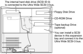
**Replacement Note:** When inserting the rear hard drive into a WS 9650, you should connect the drive to the Ultra Wide SCSI cable. The graphic at left shows the routing of the two SCSI cables in the WS 9650.
