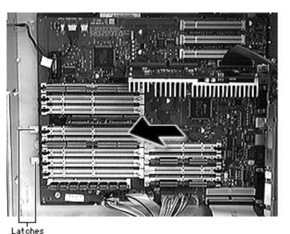
7 Release the two plastic latches on the front of the logic board.
