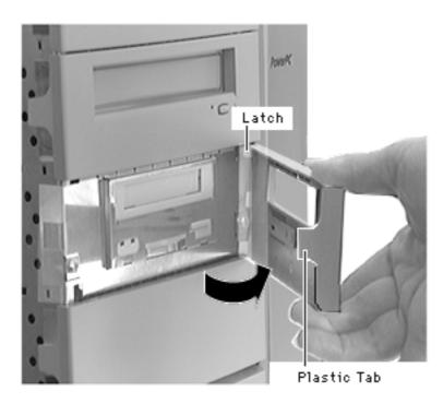
3 Swing the bezel open, and remove the bezel from the right edge of the hard drive.
