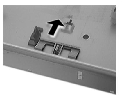
5 Slide the logic board latch forward and remove it from the computer.
