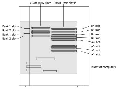
Figure: PM 8600 Series DRAM DIMM Slots
