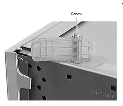
4 Remove the screw and washer and remove the lever.
