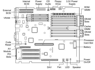
Figure: PM 8600/200 Logic Board
