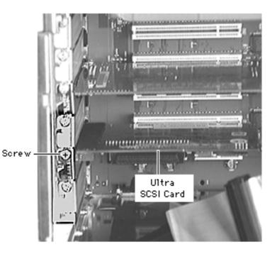
2 Using a Phillips screwdriver, remove the screw securing the Ultra SCSI card to the rear panel.
