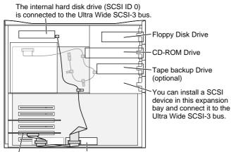
SCSI PCI Card One 5.25" Hard Disk Drive or two 3.5"Hard Disk Drives can be installed on the floor of the server and connected to the Ultra Wide SCSI-3 bus. (Some Workgroup Server models come with a second Hard Disk Drive [SCSI ID 1] installed here.)
