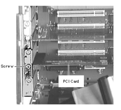
1 Using a Phillips screwdriver, remove the screw securing the PCI card to the rear panel.
