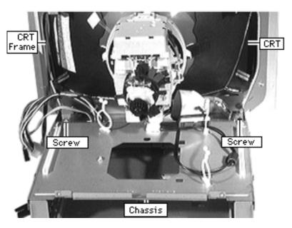
**Warning:** Support the top of the CRT. The CRT is very heavy and may fall forward as you complete this procedure.
