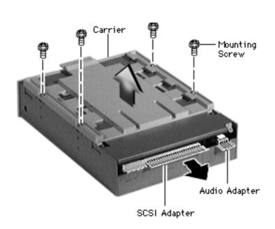
**Replacement Note:** Retain the carrier, screws, and adapters for installation on the new drive.
