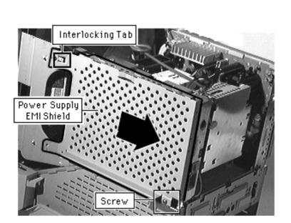
3 Slide the power supply shield back to clear the interlocking tab and remove the shield.
