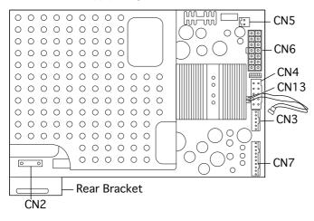
**Replacement Note:** This diagram shows the location of the rear bracket and the power supply cable connections for the original version. For Rev. B diagram, See "Power Supply, Rev. B"
