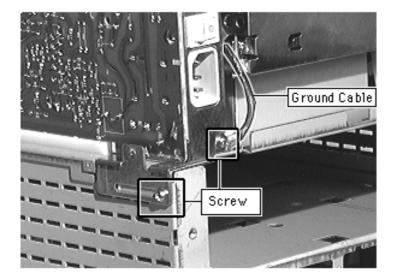
4 Remove the screw and short grounding cable from the lower rear corner of the power supply.
