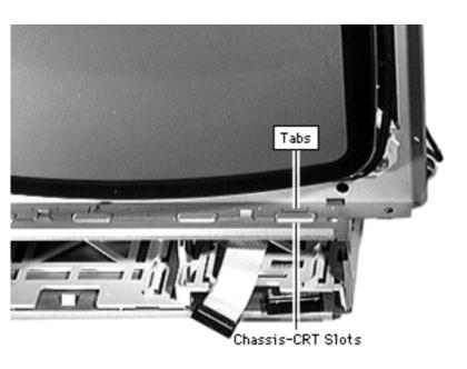
2 Pry back the metal tab from the raised slot on each side of the chassis.
