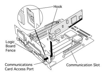
2 Angle the hook-end of the card down and bring the hook under and up through the communications card access port. The hook should rest against the outside of the logic board fence.
