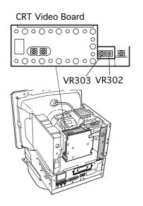
5 Using a fine-tip plastic adjustment tool, set the green gain (VR303) and red gain (VR302) controls to their middle positions.
