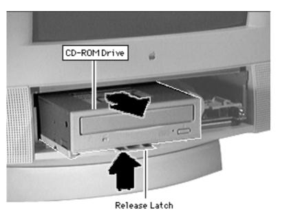
Push up the release latch and pull the CD-ROM drive from the chassis.
