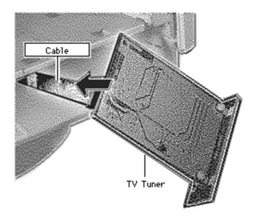
3 Disconnect the TV Tuner cable and remove the TV Tuner.
