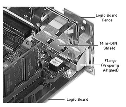
**Replacement Note:** Verify that the flange on the logic board fence is properly aligned with the mini-DIN shield.
