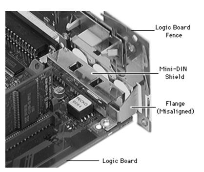
Align the flange around the mini-DIN shield first, then swing the rest of the logic board fence into place.
