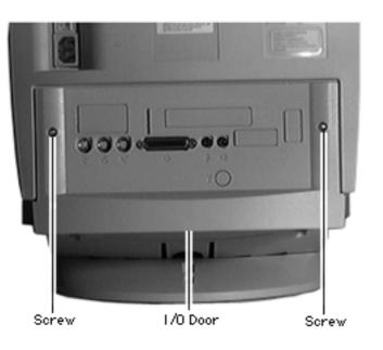
1 Remove the two security screws.
