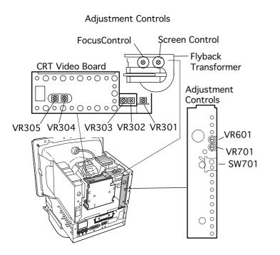
**Note:** The controls on this monitor require a small plastic Phillips-head tool or a small plastic flat-head tool to make adjustments.
