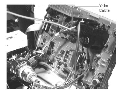
security rail and rest the analog board on the top of the chassis.
