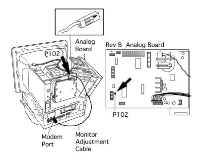
• For Rev. B, connect one end of the monitor adjustment cable to P102. The arrow mark on the plug connector (see graphic) must go over the pin closer to the top of the analog board. Hold the connector with gold connectors facing you, and place the connector on the two pins at P102.
