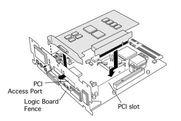
6 Press the PCI card adapter contact points into the PCI slot on the logic board.
