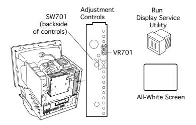
3 If necessary, use a plastic tool to reposition the arm of the horizontal centering switch (SW701).
