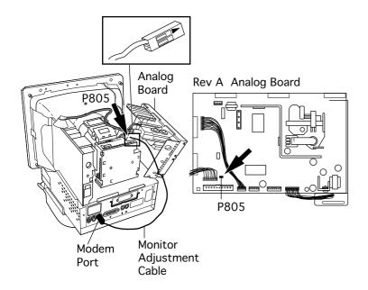
• The square silkscreened marking at P805 (Rev. A only) indicates pin 1 on the analog board. For Rev. A, connect one end of the monitor adjustment cable to P805. Be sure to position the connector so the pin 1 opening is aligned over pin 1 (square marking) on the analog board.
