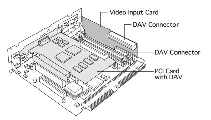
**Note:** The DAV connector on the video input card provides some of the functionality of the DAV connectors found on the Power Macintosh 7100 and 8100 models, and the Macintosh Quadra AV models, but it is not compatible with any of those connectors.
