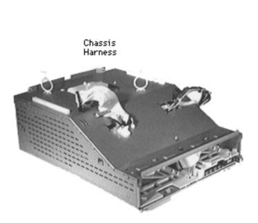
Remove the chassis/wiring harness.
