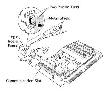
Remove the communications card access cover by pushing the two plastic tabs apart and removing the metal shield.
