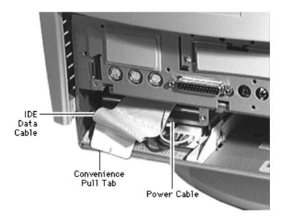
3 Using needle-nose pliers, pull up the release latch and slide the IDE hard drive from the chassis.
