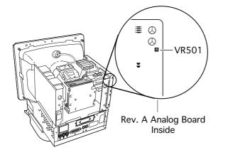
4 Using a fine-tip plastic adjustment tool, set the high-voltage adjustment control (VR501 on Rev. A, VR702 on Rev. B is pictured on next page) so the voltmeter reads 29.5 volts DC (± 0.1 volt).
