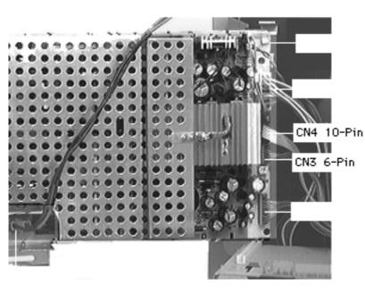
**Note:** The power supply-to-analogboard connectors are keyed and fit very tightly. You may need to use a jeweler's screwdriver to loosen the sockets of these connectors.
