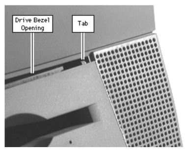
**Replacement Note:** Insert the drive bezel hinge tabs behind the upper corners of the front bezel opening. Swing the drive bezel down until it snaps closed.
