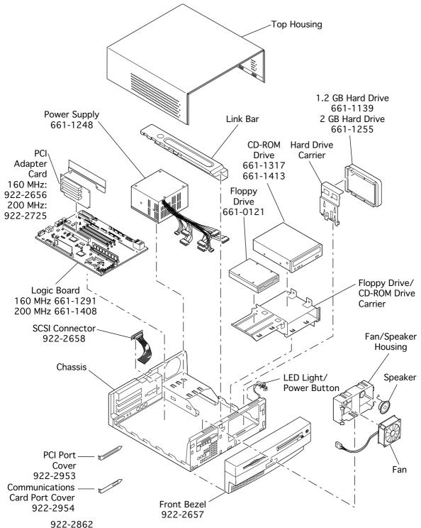
The Housing Assembly includes the Chassis, LED Light, Power Button, Fan/Speaker Housing, Fan, Speaker, Drive Carriers, Top Housing, Link Bar
