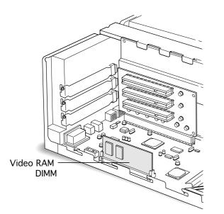
2 To install a PCI card in the bottom slot of the Power Macintosh 4400/ 160, you must temporarily remove the video RAM DIMM. Press down on the video RAM DIMM slot while pulling up on the video RAM DIMM.
