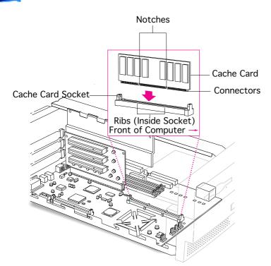
Note: The cache card is designed to fit into the slot only one way.
