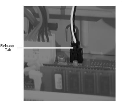
Note: Press the release tab of the soft-power connector to remove it. Grasp the plastic connector (not the wires) when removing the CD audio cable.
