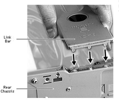
Press the rear of the bar to lock the pegs into the slots in the rear of the chassis.
