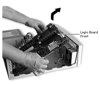
3 Raise up the front of the logic board and pull the external ports out of the access holes in the rear of the chassis. Guide the logic board away from the power supply.
