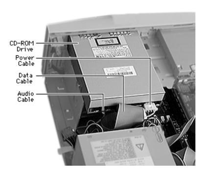
1 **Note:** Press the plastic release tab on the audio tab to remove it.
