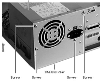
3 Remove the 4 screws that secure the power supply to the rear of the chassis.
