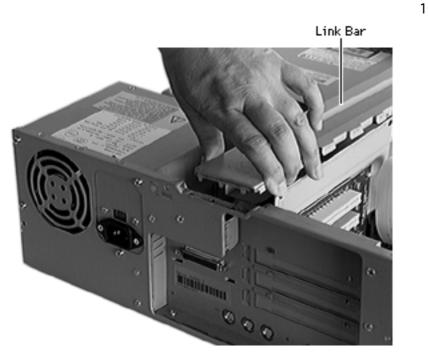
Detach the pegs of the link bar from the slots in the rear of the computer.
