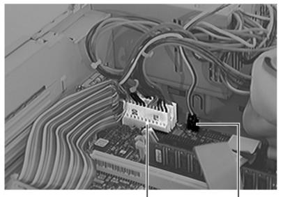
Disconnect the five power supply cables from the logic board sockets.
