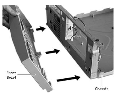
**Replacement Note:** Insert the three tabs at the front base of the chassis. Snap the release tabs into place.
