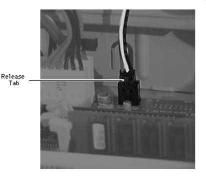
1 **Note:** Press the release tab of the soft-power connector to remove it.
