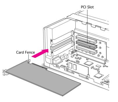
4 Insert the PCI card into the PCI slot, aligning any ports on the card with the port access opening. Press the card firmly into the slot.
