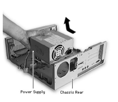
4 Push the power supply about one cm from the rear of the chassis and lift it out of the computer.
