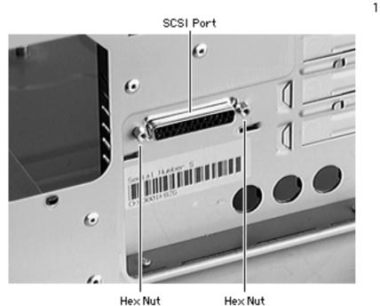
Remove the two hex nuts that secure the SCSI cable to the rear of the chassis.
