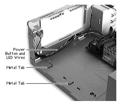
Replacement Note: Be sure the power button and LED wires are firmly held under the clips and clear of the floppy/CD-ROM carrier path. These wires are easily cut when the drive carrier slides across them. Also pull the power supply wires out of the way. Guide the CD-ROM drive under the metal spring tabs at the top of the opening in front of the chassis. Align the carrier with the metal tabs at the base of the chassis and slide the carrier toward the chassis front until it fits
