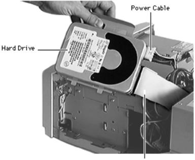
2 Disconnect the power and data cables attached to the hard drive.
