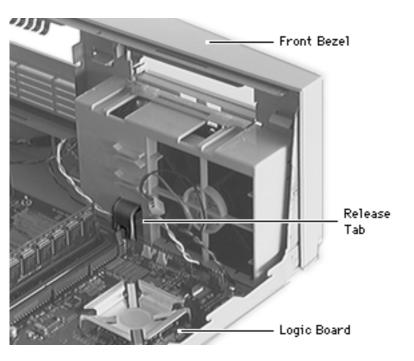
2 Press the release tab near the front panel to release the logic board.
