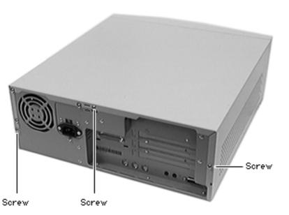
1 Remove the screws that secure the housing to the rear of the chassis.
