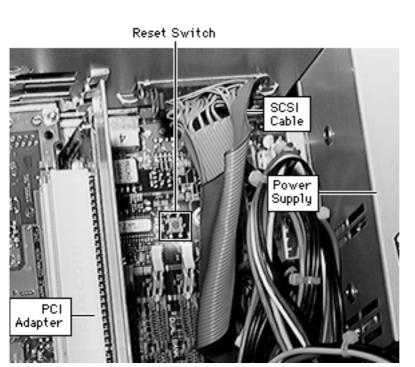
4 Press the reset switch on the logic board using a flat plastic tool.
