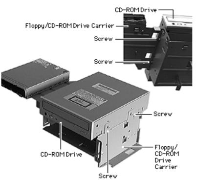
**Note:** A long-neck Phillips screw driver will make it easier to remove the CD-ROM screws under the floppy carrier.
