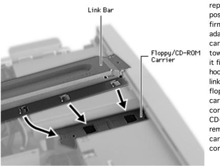
Replacement Note: To replace the link bar, position the bar so that it firmly holds the PCI adapter board and disk drive carriers. Slide the link bar toward the front panel until it fits into place. The three hooks at the bottom of the link bar must catch the floppy/CD-ROM drive carrier. If it doesn't fit correctly after the floppy/ CD-ROM drive carrier was removed, make sure the carrier was installed correctly.
