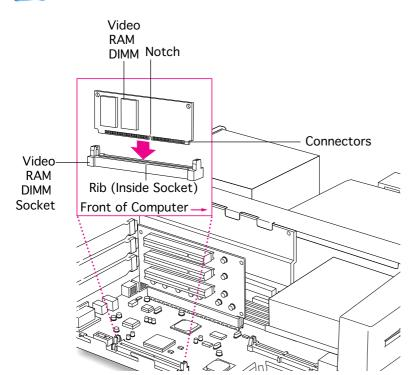
Note: Do not touch the video RAM DIMM connectors. Handle only by the edges.
