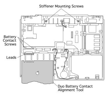
**Note:** If leads 1 or 5 flex or offer resistance to the alignment tool, perform the following steps. If there is no resistance, the contacts are aligned.
