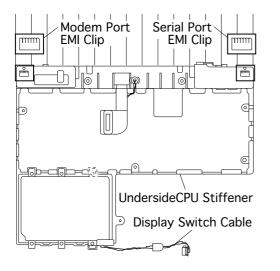
Important: Check that the serial port EMI clip is attached to the bottom of the CPU stiffener. If it is missing, replace the stiffener. On international units, also replace the stiffener if the modem port EMI clip is missing.
