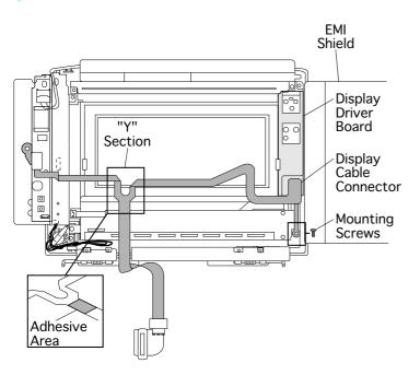
4 Using a T-8 torx driver, remove the lower right mounting screw from the display cable.
