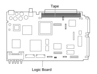
2 Raise the side of the logic board opposite the 152pin docking connector. Slide the docking connector out of the bottom case and remove the logic board.
