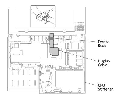
**Caution:** PowerBook Duo cables are fragile and easily torn or damaged. Handle all cables with care.
