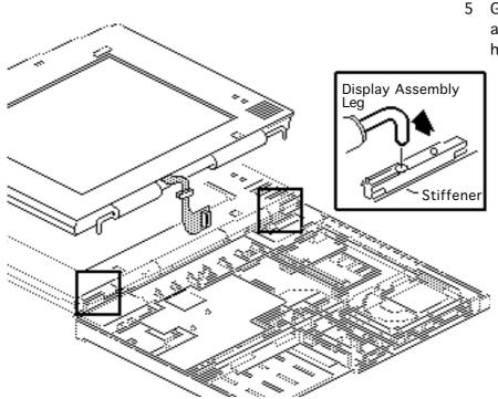
5 Gently lift the display assembly legs out of the holes in the stiffener.
