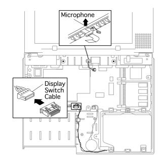
1 Pull the display switch ferrite bead off the bottom case.
