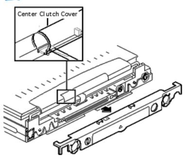
**Caution:** The display cable, which is fragile, is under the left side of the center clutch cover. Be careful not to damage the display cable with the screwdriver.
