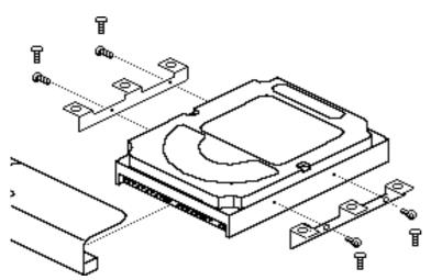
**Note:** Remove the mounting brackets and cable only if you are returning a defective drive to Apple.
