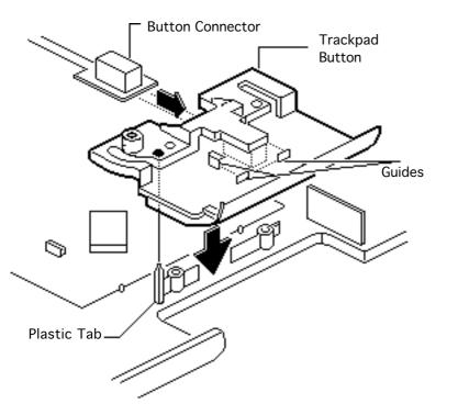
**Replacement Note:** Install the trackpad button before installing the trackpad carrier: Slide the button connector into the guides on the button. Line up the button's lower left hole with the plastic tab on the top case and set the button in place.
