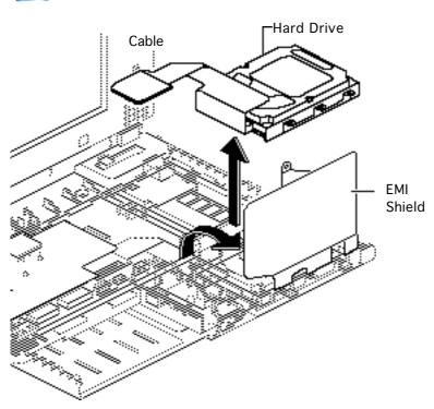
3 Pull back the EMI shield and lift out the hard drive.
