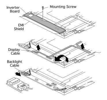
1 Using a T-8 torx driver, remove the inverter board mounting screw.
