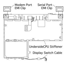
**Important:** Check that the serial port EMI clip is attached to the bottom of the CPU stiffener. If it is missing, replace the stiffener. On international units, also replace the stiffener if the modem EMI clip is missing.
