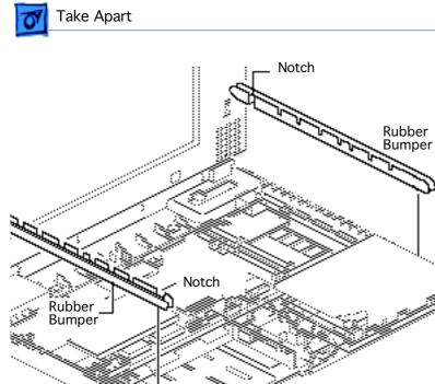
4 Remove the two rubber bumpers from the chassis.
