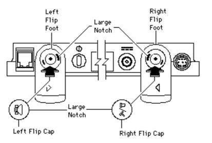
**Replacement Note:** The left and right foot caps are not interchangeable; neither are the flip feet. Note the icons on each and install them with notches aligned as shown.
