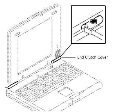
Using a jeweler's flat-blade screwdriver, push off the left and right end clutch covers.
