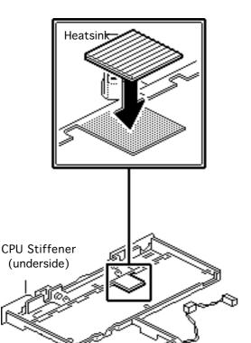
**Note:** Replacement CPU stiffeners include the rear cover, I/O door, feet, display switch, and heatsink. You can also individually replace the rear cover, I/O door, and feet.
