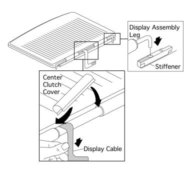
**Replacement Note:** (For display assembly only) Before reattaching the display assembly to the PowerBook Duo, install the center clutch cover.
