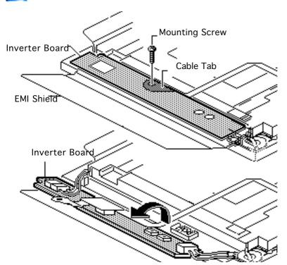
1 Using a T-8 torx driver, remove the inverter board mounting screw.
