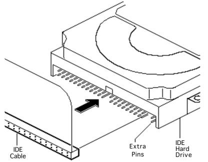
**Replacement Note:** IDE and SCSI cables are not interchangeable. If you replace a cable, make sure you install the correct one.
