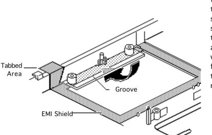
**Replacement Note:** If the trackpad EMI shield is twisted, replace it. Gently slide the top portion of the shield into the groove on the top case. Be sure the tabbed area is unbent; bending would prevent the shield from making contact with the CPU stiffener after reassembly.
