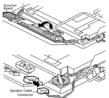
2 Lift up the inverter board and carefully turn it on its left side to expose the cable connectors.
