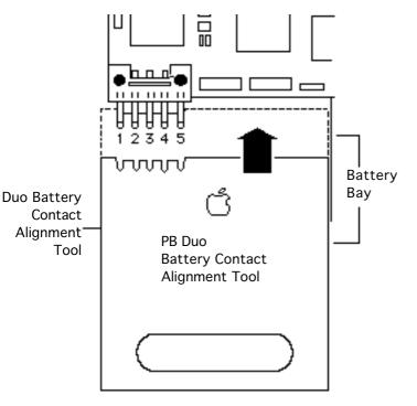
**Note:** Perform the battery contact alignment procedure when you replace a Power-Book Duo logic board or when a known good battery has power problems. (Also see "Troubleshooting Info: **Battery Contact** Alignment.") Use the Duo battery contact alignment tool to align the two outer battery contacts so they are perpendicular to the edge of the logic board.
