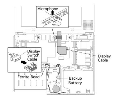
**Note:** It is unnecessary to disconnect the backup battery in this next step.
