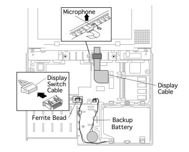
3 Using a jeweler's flatblade screwdriver, carefully disconnect the display switch cable.
