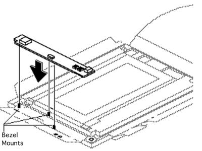
**Replacement Note:** Place the inverter board onto its three plastic bezel mounts.
