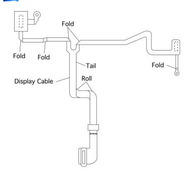
6 Gently peel the "Y" section of the display cable from the display.
