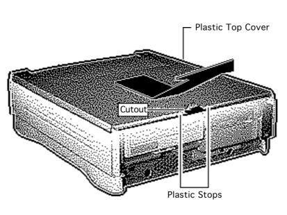
Caution: When using a screwdriver to release a latch, be careful not to scratch or gouge the plastic.
