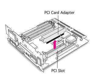
6 Pull up on the PCI card adapter to remove it from the PCI slot.
