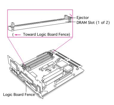
1 Push the ejector on the DRAM slot outward and down to open it.
