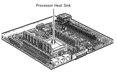
Replacement Note: You must remove the heat sink of the 6300 Series logic board to install or replace a SIMM in the slot next to the processor.
