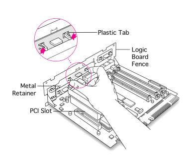
3 If the PCI card has ports for connecting equipment, remove the plastic access cover from the logic board fence. On the inside of the logic board fence, squeeze together the two plastic tabs of the plastic access cover.
