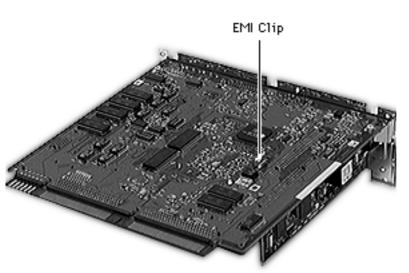
Caution: Take care to avoid compressing the EMI clip on the bottom of the logic board. If possible, support the underside of the board to avoid compressing the EMI clip.
