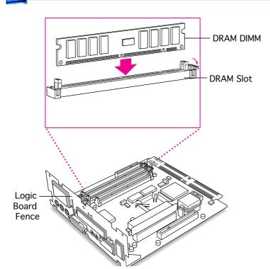
Caution: Do not touch the DIMM's connectors. Handle the DIMM only by the edges.
