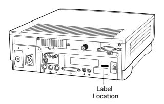
37 Apply the REA label (part number 922-2396) to the left of the communication port on the back of the unit.
