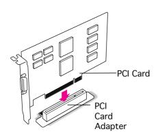
8 Press the PCI card connector into the PCI card adapter.
