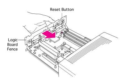
4 Note: The reset button is located in a different place on the 6320 and 6360 logic boards. See the diagrams on this page and the next page.
