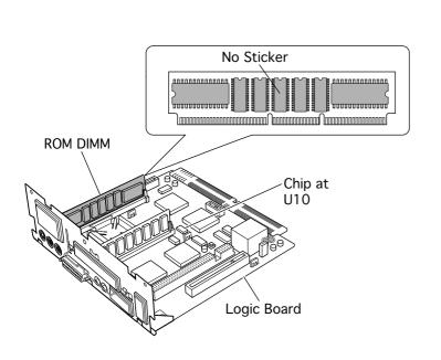
Inspect the clock chip at location U10. If it is **not** printed with part number 343S1191 or 343S1121 (ignore any letters following the part number), replace the logic board. **Go to step 14.**
