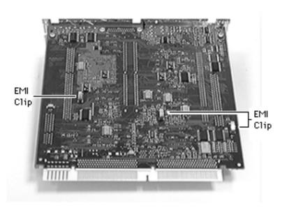
Caution: Take care to avoid compressing the EMI clips on the bottom of the logic board. If possible, support the underside of the board to avoid compressing the three silver-colored EMI clips.
