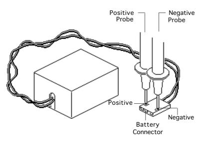
Set the voltmeter to the 10 VDC scale.
