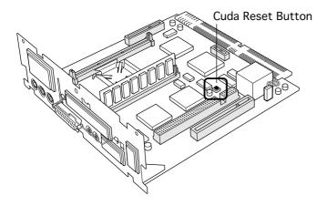
**Note:** The reset button is located in a different place on the 6320 and 6360 logic boards. See the diagrams on this page and the previous page.
