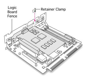
11 Replace the retainer clamp inside the logic board fence.
