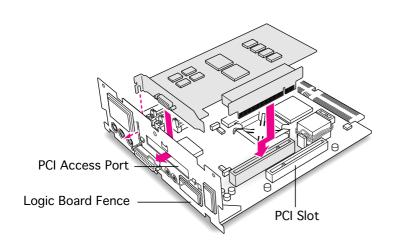
9 Press the PCI card adapter contact points into the PCI slot on the logic board.
