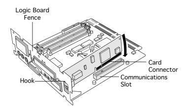
7 Insert the card connector into the communications slot.
