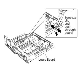
30 With the logic board facing right side up, squeeze together the top of each EMI clip and push it out through the slot.
