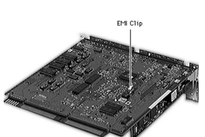
Caution: Take care to avoid compressing the EMI clip on the bottom of the logic board. If possible, support the underside of the board to avoid compressing the silver-colored EMI clip.
