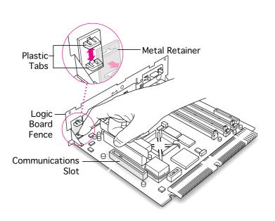
Remove the communications card access cover by pushing the two plastic tabs apart and removing the metal retainer.
