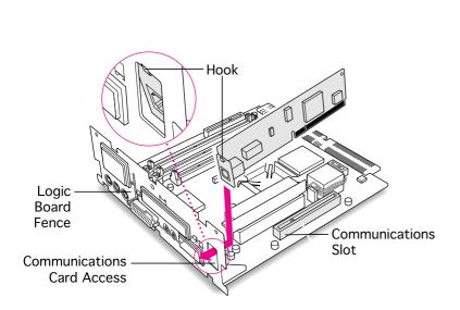
Angle the hook-end of the card down and bring the hook under and up through the communications card access port. The hook should rest against the outside of the logic board fence.
