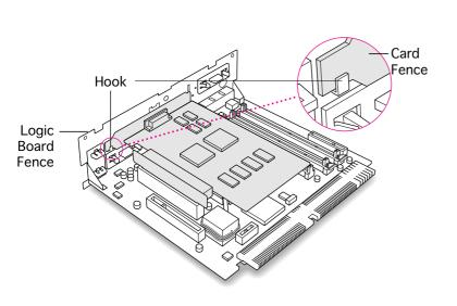
10 Be sure the PCI connector is in the access port and accessible outside the logic board fence.
