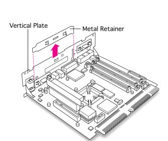
5 Remove the metal retainer from inside the logic board fence.
