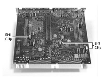
Caution: Avoid compressing the EMI clips on the bottom of the logic board. If possible, support the underside of the board to avoid compressing the three silver-colored EMI clips.
