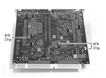
Caution: Take care to avoid compressing the EMI clips on the bottom of the logic board. If possible, support the underside of the board to avoid compressing the three silver-colored EMI clips. (The Performa 6360/160 has only one EMI clip.)
