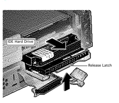
3 **Caution:** When using a screwdriver to release a latch, be careful not to scratch or gouge the plastic.
