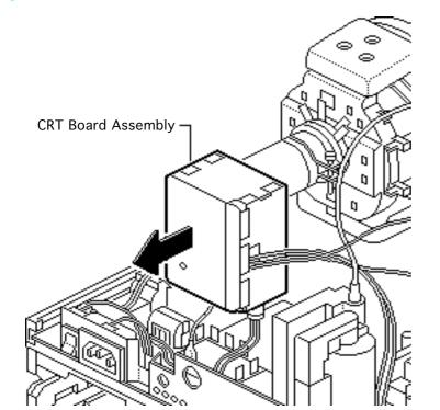
**Caution:** Twisting, bending, or applying force to the video board assembly could damage the neck of the CRT. Be sure to pull the CRT board assembly straight off the CRT.
