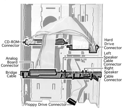
Stand at the front of the chassis, looking down at the top of the chassis, and disconnect the following in the order listed: analog board connector, CD-ROM drive connector, and hard drive connector. (The connector tabs operate much like largescale SIMM slot connectors on logic boards.)
