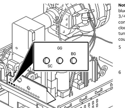
**Note:** To set the green and blue drive controls to their 3/4 position, turn the controls to their full clockwise position and then turn back 1/4 turn counterclockwise.
