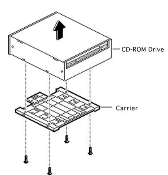
3 Remove the four mounting screws and remove the CD-ROM drive from the carrier.
