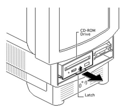
1 Pull up the latch and pull out the CD-ROM drive.
