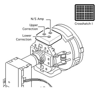
Using a hex-head plastic adjustment tool, adjust the N/S amp control for best convergence of horizontal lines at the top and bottom of the screen.
