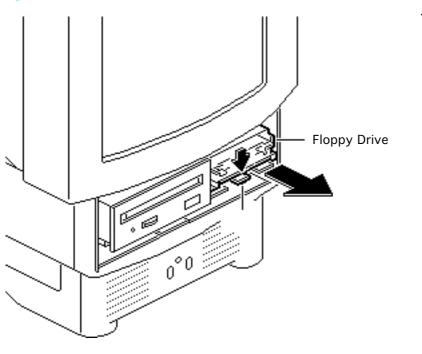
1 Push down the latch and pull out the floppy drive.
