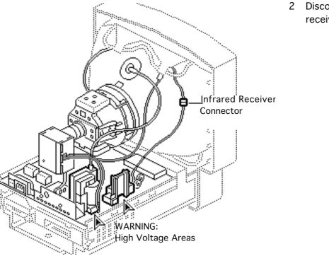
2 Disconnect the infrared receiver connector.
