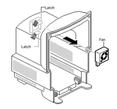
Push out the two latches and remove the fan assembly.
