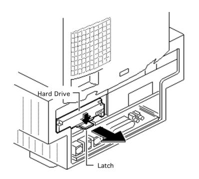
1 Push down the latch and remove the hard drive.
