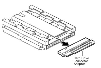
2 Pull out the hard drive connector adapter.
