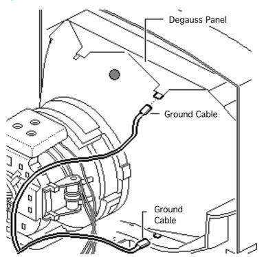
1 Disconnect the two ground cables from the degauss panels.
