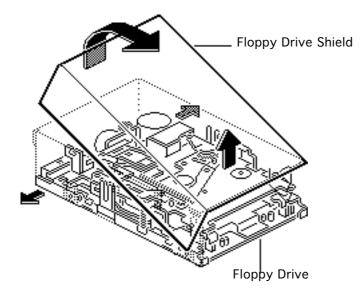
5 Pull out the sides of the floppy drive shield, lift the back of the shield, and remove it from the floppy drive.
