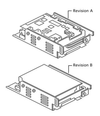
Replacement Note: If you are replacing a defective Hard Disk 20SC, be aware that Apple currently ships Revision A and Revision B versions of this hard drive and each version must be replaced like-for-like. To differentiate between drive versions, check their circuit boards. For Revision A drives, the component side of the board is up; for Revision B drives, the solder side of the board is up. For part numbers, refer to the Service Source parts database.
