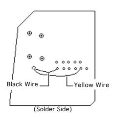
Replacement Note: Some replacement fans have a black wire and a yellow wire that must be soldered to the back side of the analog board. Insert these wires through the arrow clip hole in the board and solder them to the points shown.
