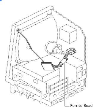
Replacement Note: If you receive a replacement analog board that is packaged with a ferrite bead, and if the customer's video cable does not have a ferrite bead attached, install the packaged ferrite bead on the video cable as shown. Secure the ferrite bead to the cable with a tie-wrap.
