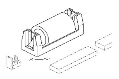
**Replacement Note:** When replacing the new battery, orient it so that the end marked +/ matches the +/ on the logic board.
