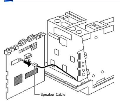
4 Disconnect the speaker cable from the logic board.
