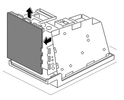
Slide up the logic board until its tabs are aligned with the notches in the chassis. Swing out the right side of the board and remove it from the chassis.
