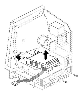
Remove the two mounting screws and lift out the hard drive with carrier attached.
