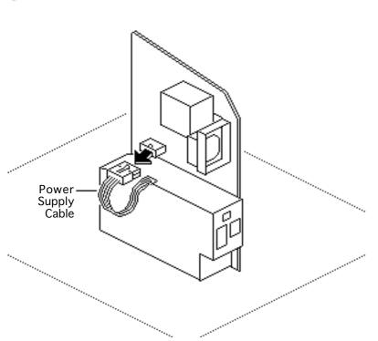
Place the analog board on a protective pad and disconnect the power supply cable.
