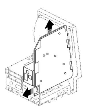
Caution: When removing the analog board, be careful not to catch the brightness control knob on the chassis and not to bump the neck of the CRT.
