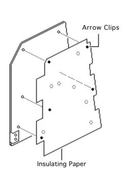
1 Compress the arrow clips and remove the insulating paper from the analog board.
