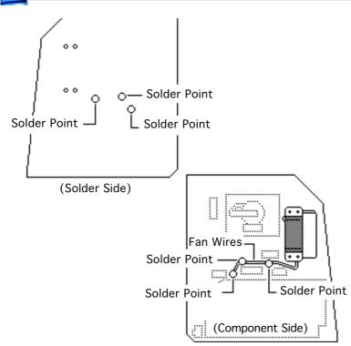
2 Check the front and back of the analog board for wires connecting the fan to the board. Desolder these wires at their solder points at the back of the analog board.
