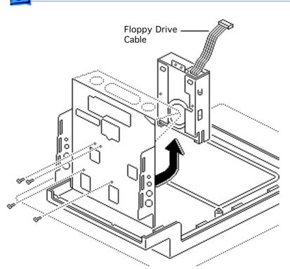
Remove the four mounting screws and lift out the lower floppy drive. Disconnect and keep the floppy drive cable.
