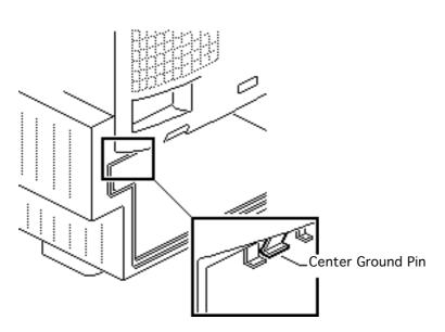
Note: If the rear cover has bronze tape on the rear cover shield, remove the tape before removing the rear cover. Bend back the center ground pin on the rear cover shield about 1/8 inch. Do not replace the bronze tape.
