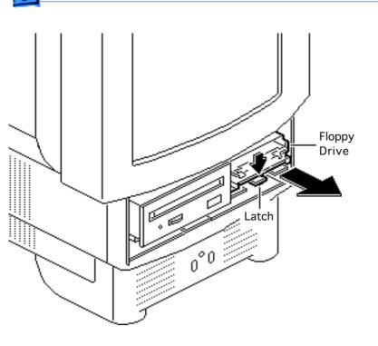
Push down the latch and pull out the floppy drive.
