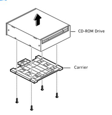
Remove the four mounting screws and remove the CD-ROM drive from the carrier.
