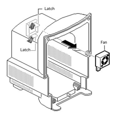
Push out the two latches and remove the fan assembly.
