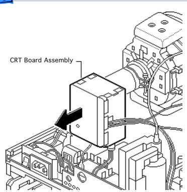
5 **Caution:** Twisting, bending, or applying force to the video board assembly could damage the neck of the CRT. Be sure to pull the CRT board assembly straight off the CRT.
