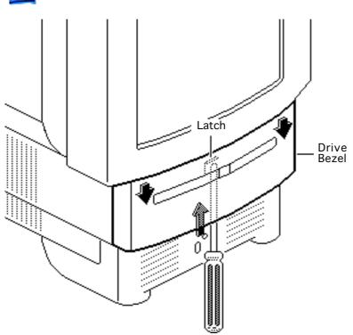
Using a flat-blade screwdriver, push up the latch. Pull down and remove the drive bezel.
