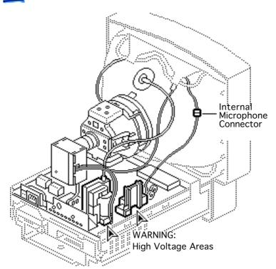
Disconnect the internal microphone connector.
