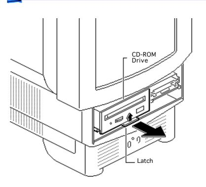
Pull up the latch and pull out the CD-ROM drive.
