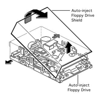
Pull out the sides of the floppy drive shield, lift the back of the shield, and remove it from the floppy drive.
