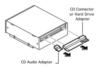
Pull out the CD connector adapter and the CD audio adapter.
