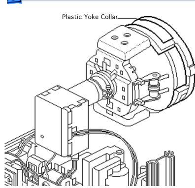
With one hand, grasp the plastic yoke collar and rotate it until the top and bottom edges of the picture are parallel with the top and bottom of the bezel.
