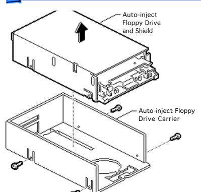
Remove the four mounting screws and remove the floppy drive from the carrier.
