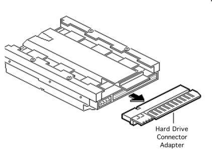
2 Pull out the hard drive connector adapter.
