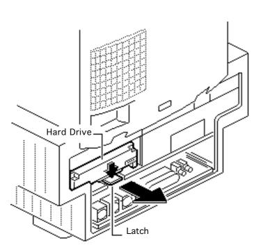
1 Push down the latch and remove the hard drive.
