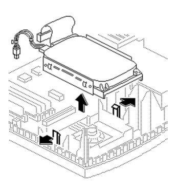
Release the two tabs and lift the drive (along with its carrier) out of the computer.
