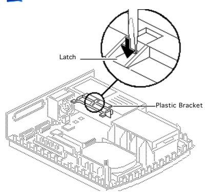
3 To remove the plastic bracket, press on the latch with a screwdriver and lift the bracket from the power supply.
