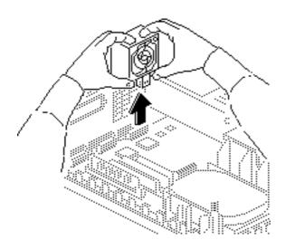
Place your thumbs under the fan and using some force pull up until the fan snaps free.
