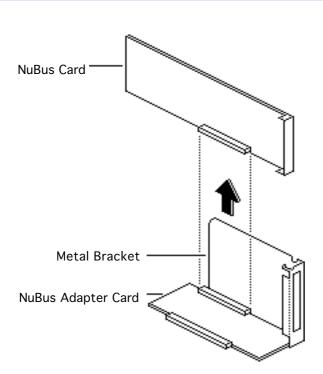
3 If you are replacing the NuBus card, place the adapter card on a flat surface, and carefully pull the NuBus card from the adapter card connector.
