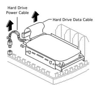
I Disconnect the hard drive power cable and hard drive data cable from the logic board.
