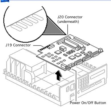
4 Caution: Be sure the power on/off button clears the rear panel before you lift the logic board out of the case. While lifting the board, do not touch connector J19 or J20. (The oil from your skin harms the connectors.)
