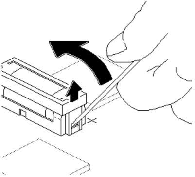
screwdriver, pry open the latch at the end of the holder and lift off the cover.
