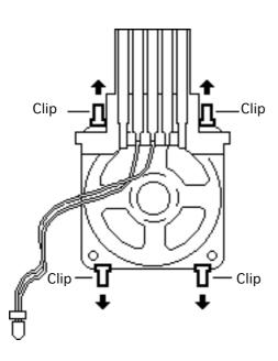
Release the four clips and lift the speaker out of the case.
