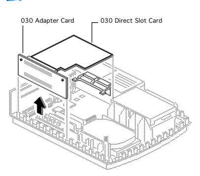
1 Pull straight up on the adapter card and carefully remove it and the direct slot card from the logic board.
