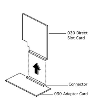
2 If you are replacing the direct slot card, place the adapter card on a flat surface, and carefully pull the direct slot card from the adapter card connector.
