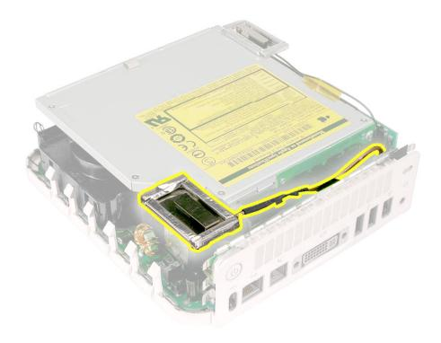
6. Using the black stick push the black latch (see inset) toward the I/O ports to release the antenna from the internal frame.
