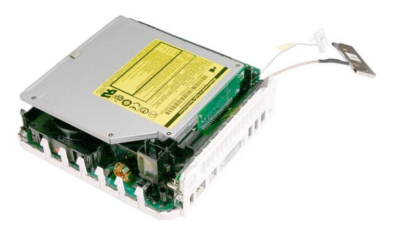
9. With a jeweler's # 0 Phillips screwdriver remove three screws on the internal frame.
