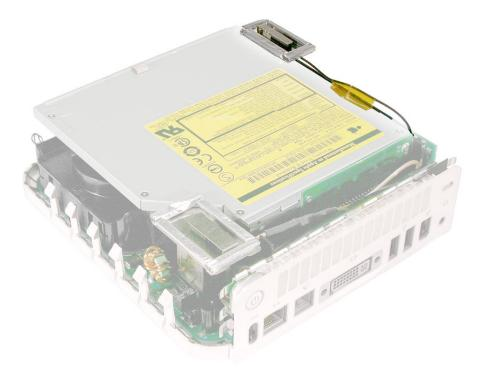
7. Pull the Bluetooth antenna up and out of the openings on the plastic rail. Free the antenna cable from the kapton tape. **Important:** Take care handling the Bluetooth antenna as a bent or warped antenna will affect Bluetooth connectivity.
