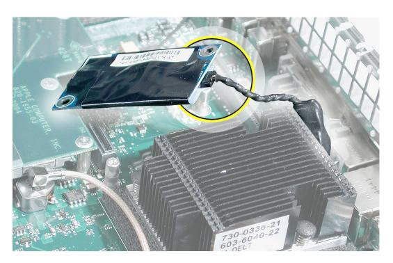
2. Using a jeweler's #0 Phillips screwdriver, replace the two modem screws.
