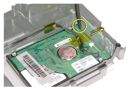
With the gold pins on the interconnect board facing up, press the interconnect board onto the hard drive and optical drive connectors. Replace the optical drive screws (circled). Caution: Be careful not to bend the hard drive pins when connecting the interconnect board.
