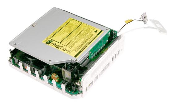
9. Free the power button cable from the kapton tape on the internal frame.
