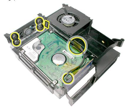
2. With your finger or black stick, pry the speaker off the internal frame. **Note:** Watch that the rubber grommets for the speakers don't fall off as you remove the speaker.
