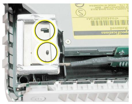
9. Secure the power button cable to the internal frame with the kapton tape.
