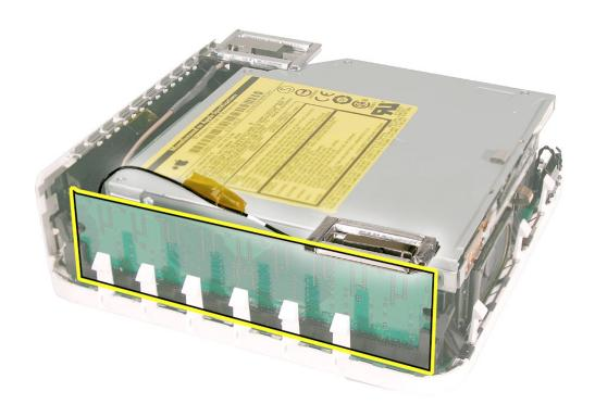
Remove the Bluetooth antenna and the kapton tape. Important: Take care handling
