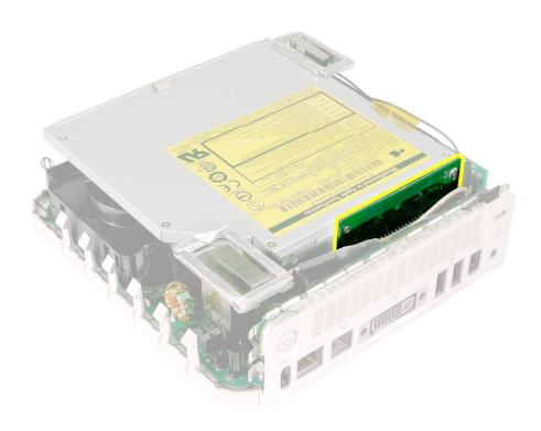
1. Locate the interconnect board. Using a a jeweler's #0 Phillips screwdriver, remove the two screws.
