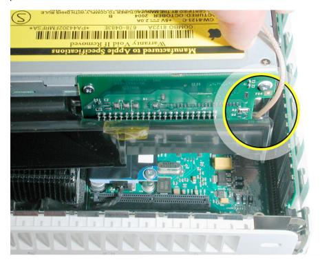
23. Replace the three screws on the internal frame.
