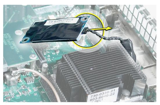
2. Turn over the logic board. Using a black stick, push the RJ-11 connector off the logic board.
