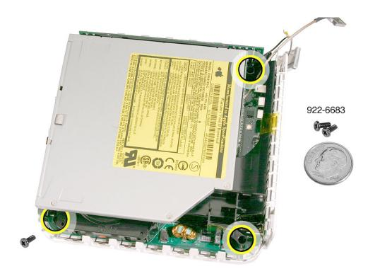
11. Lift the internal frame straight up.
