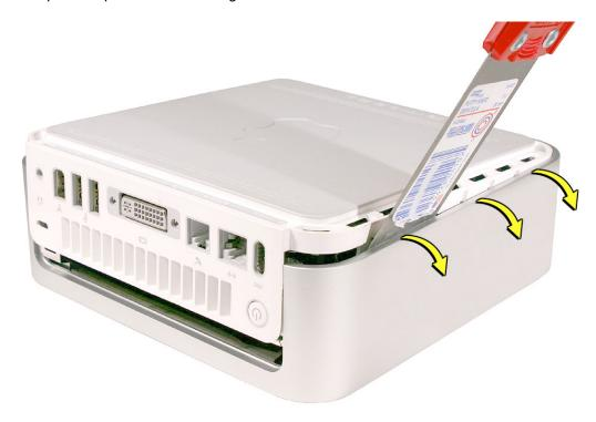
11. Push the I/O panel upward until the top housing is removed. The popping sounds will continue as you push the I/O panel; this is normal.
