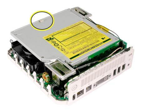
3. Replace the four optical drive screws.
