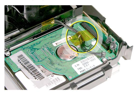
6. With a black stick or other nonconductive tool, pry the hard drive off the connector on the interconnect board. Lift the hard drive out of the internal frame and set it aside.
