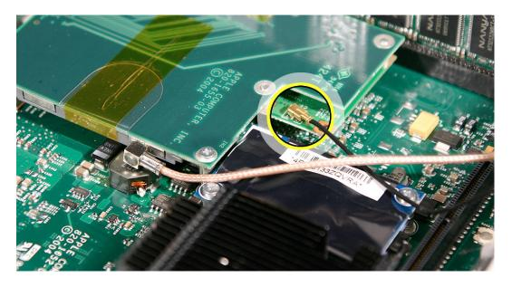
13. Remove the two screws on the mezzanine board. Lift the mezzanine board straight up and off the logic board connector. **Caution:** The AirPort antenna cable is still attached to the mezzanine board. Remove the AirPort antenna cable if required to perform the repair.
