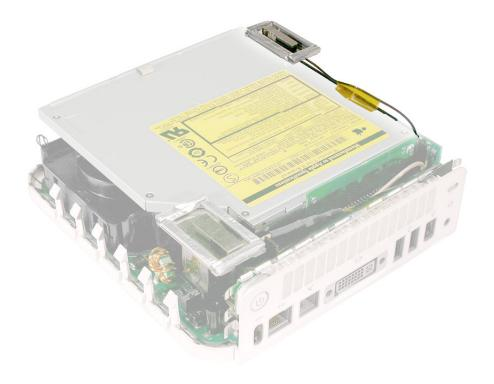
3. Pull the Bluetooth antenna up and out of the openings on the plastic rail. Free the antenna cable from the kapton tape. **Important:** Take care handling the Bluetooth antenna as a bent or warped antenna will affect Bluetooth connectivity.
