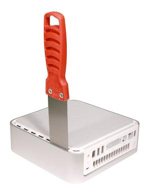
4. Gently release the internal latches by prying the tool away from the computer.
