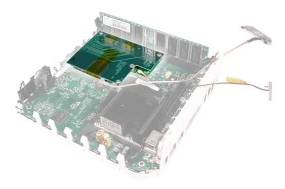
15. To access the AirPort Extreme card remove the two screws on the mezzanine board with a jeweler's # 0 Phillips screwdriver. Pull the mezzanine board straight up and off the logic board connector.
