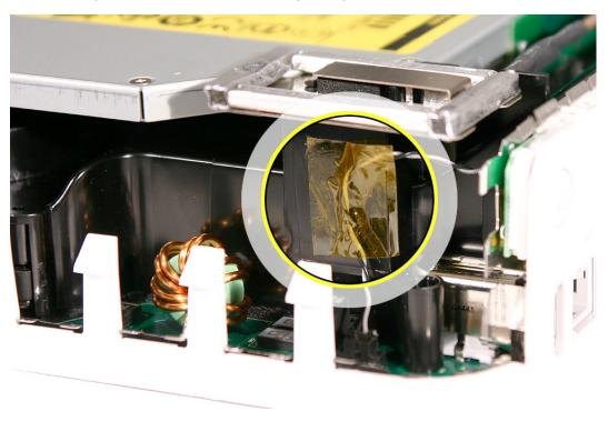
15. Lift the internal frame straight up and set it aside.
