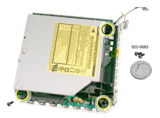
Replace the Bluetooth antenna and secure the antenna cable with kapton tape.
