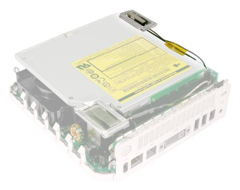
2. Pull the Bluetooth antenna up and out of the openings on the plastic rail. Free the antenna cable from the kapton tape. **Important:** Take care handling the Bluetooth antenna as a bent or warped antenna will affect Bluetooth connectivity.
