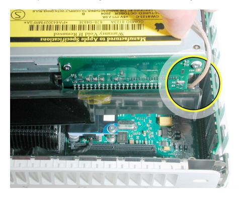
5. Replace the three screws on the internal frame.
