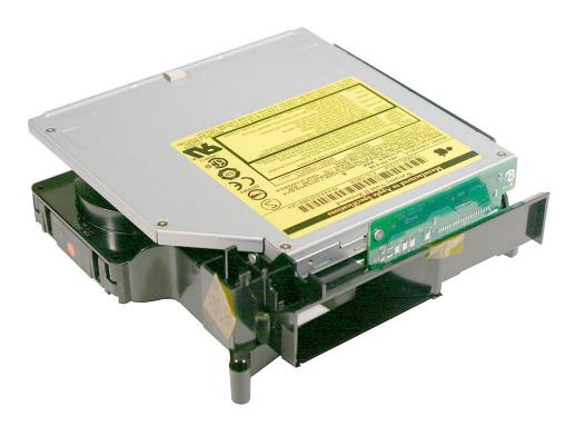
2. Hold the internal frame over the logic board as shown. Route the AirPort and Bluetooth antenna cables up through the opening in the internal frame.
