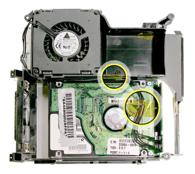
3. Replace two screws and connect the fan and speaker cables to the interconnect board.
