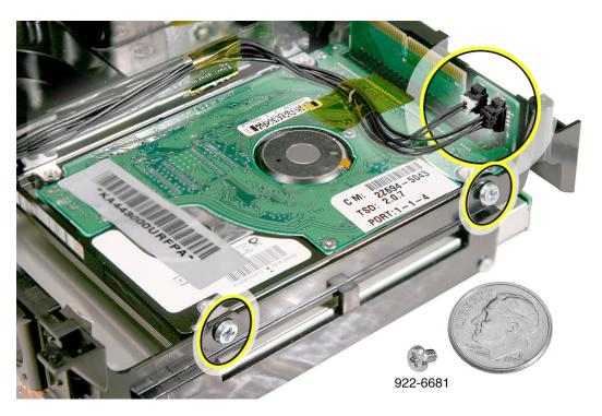
5. Remove the kapton tape to release the cables.
