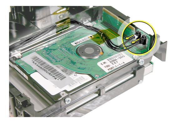
3. With a black stick or other nonconductive tool, slightly pry the interconnect board off hard drive pins. With your fingers wiggle the interconnect board off the hard drive pins. **Caution:** Be careful not to bend the hard drive pins.
