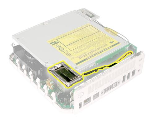
5. Using the black stick push the black latch (see inset) toward the I/O ports to release the antenna from the internal frame.
