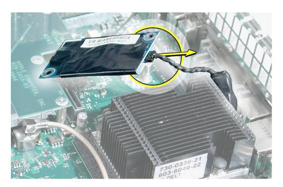
1. Connect the RJ-11 cable to the modem board.
