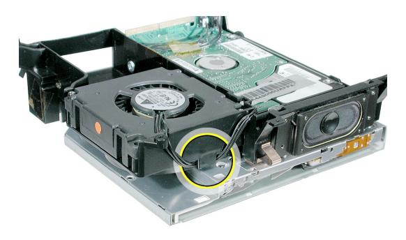
4. Remove the tape securing the fan and speaker cables.
