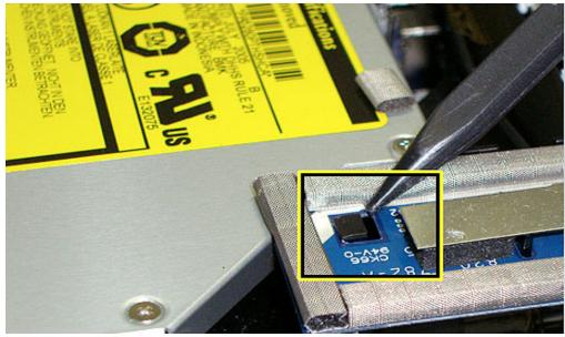
28. Secure the power button cable to the internal frame with the kapton tape.
