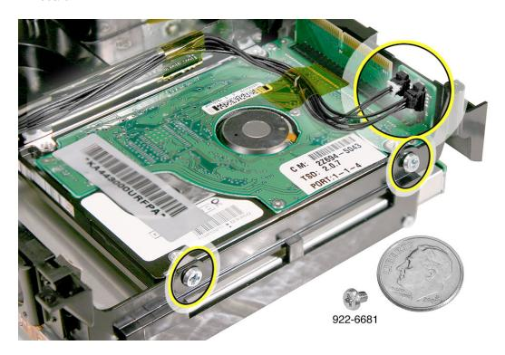
4. Replace the two hard drive screws on the inside of the internal frame.
