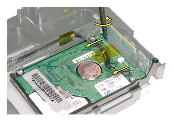
1. With the colored side of the hard drive face up, place the hard drive into the internal frame and connect it to the black connector on the interconnect board.
