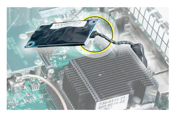
8. Connect the modem to the modem connector on the logic board, and install the two modem mounting screws.
