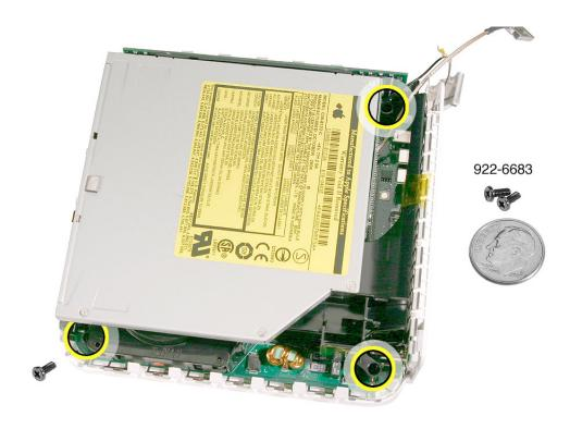
10. Lift the internal frame straight up.
