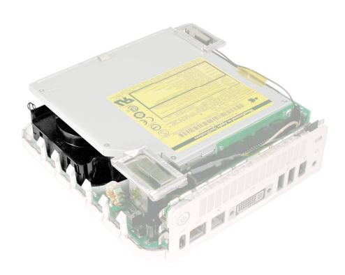
1. Turn over the internal frame to locate the fan. Remove the three fan screws with a jeweler's #0 Phillips screwdriver.
