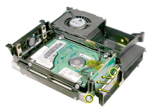
2. Connect the speaker cable (on the left) and fan cable (on the right) to the interconnect board.
