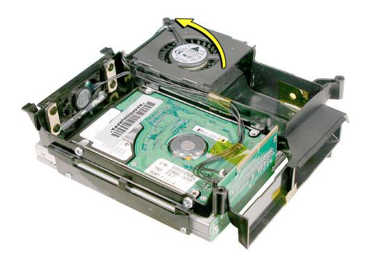
5. Using a #2 Phillips screwdriver, remove the two hard drive screws (shown by the dotted line) on the internal frame. You may need an angled screwdriver to access the screw on the right. Important: Don't remove the kapton tape from the internal frame near the screw on the right. The hole is covered to direct airflow within the internal frame.
