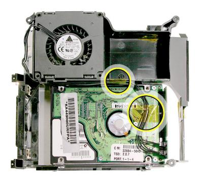
4. Free the fan cable (top cable) from another clip on the inside of the internal frame.
