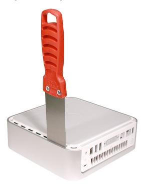
9. Gently release the internal latches by prying the tool away from the computer.
