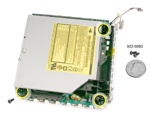
11. Lift the internal frame straight up.
