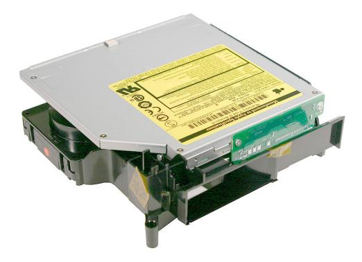
5. Hold the internal frame over the logic board as shown. Route the AirPort and Bluetooth antenna cables through the opening in the internal frame.
