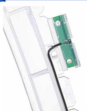
Important: Note how the antenna wire is routed through the side panel before removing. A close-up view of the right panel antenna is shown here.
