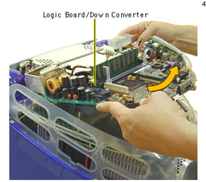
Gently lift the down converter board and logic board out of the computer.
