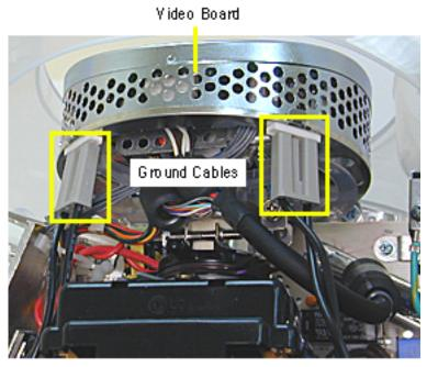
11. Disconnect the two ground cables on the video board.
