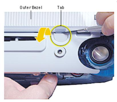
2. After removing the tabs, remove the screws located under the tabs.
