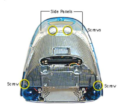
On the rear of the side panels, remove four screws. These screws connect the side panels to the divider panel (the metal chassis).
