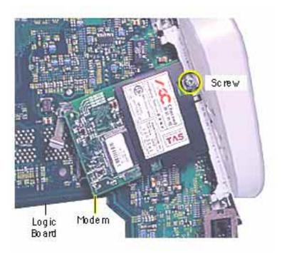
3. Turn the logic board to the underside and remove the modem screw.
