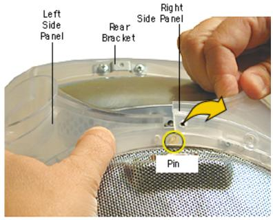
At the top rear of the side panels, pull each side panel off the plastic pin.
