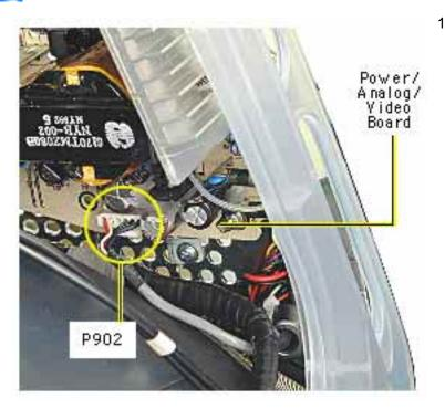
10. At the very bottom of the power/analog/video board, near the bottom of the CRT, disconnect P902, which is part of the audio/headphone/ LED/speaker cable assembly.
