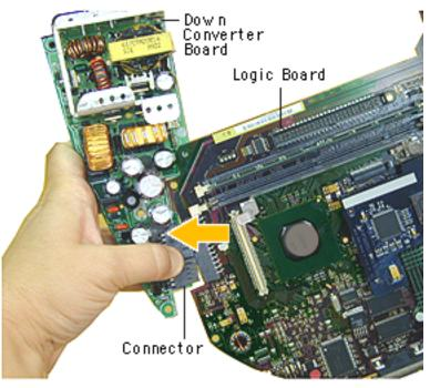
Holding onto the down converter, press down on the black connector to separate the down converter board from the logic board.
