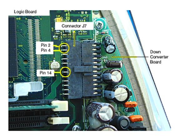
Testing Voltages at J7 on the Logic Board
