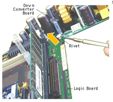
Using a flatblade screwdriver, pry the plastic rivet off the board.
