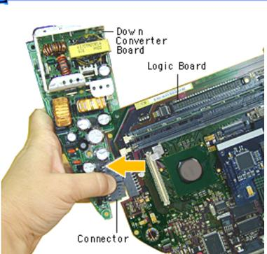
Holding onto the boards, press down on the black connector and separate the down converter board from the logic board.
