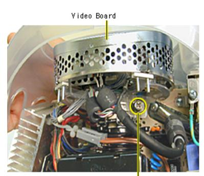
12. Loosen the CRT neck clamp screw.
