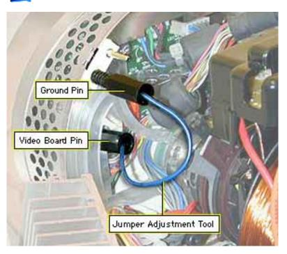
Connect one end of the jumper adjustment tool (922-4165) to the video board pin.
