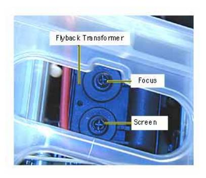
4. Adjust the focus control on the flyback transformer until the focus test pattern reaches the best frontof-screen performance.
