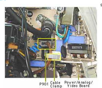
On the other side of the CRT neck, disconnect the brown degauss cable, P901, from the power/ analog/video board. Remove P901 from the cable clamp.
