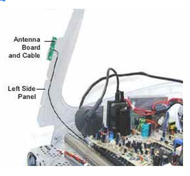
Carefully remove the antenna from the left side panel. Refer to the next page for a close up of the antenna in the left side panel.
