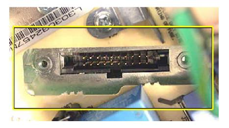
**Figure 4 Main Logic Board Connector Pins**
