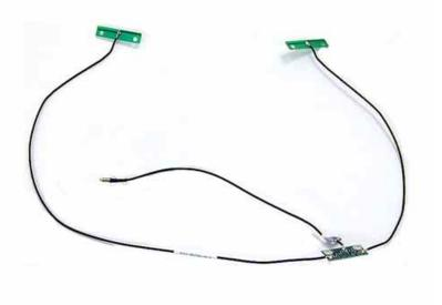
Remove the antenna board from the divider panel.
