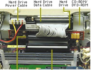
Logic Board Cable Connector **Note:** Remove SDRAM to make cable removal easier.
