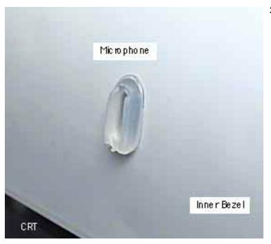
Check that the microphone protrudes through the inner bezel hole.
