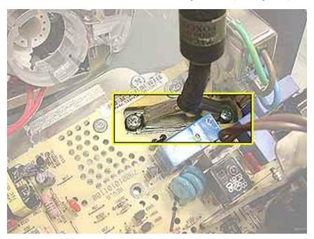
Figure 3 RGB Cable Connection
