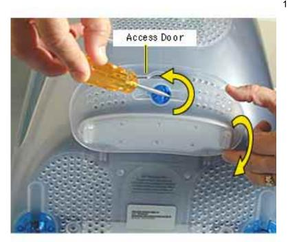
With a flatblade screwdriver or coin, turn the colored latch to open the access door.
