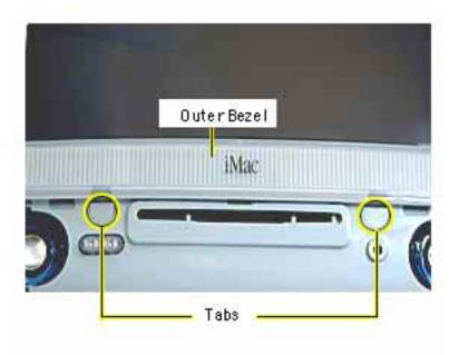
1. With a jeweler's screwdriver, carefully remove the two tabs on the front outer bezel. Refer to the next graphic for a close-up of the tab removal.
