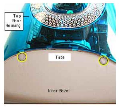
1. Remove the two tabs (screw caps) on the top inner bezel. Refer to the next page for a close-up of the tab removal.
