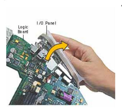
Rotate the logic board face up again and carefully slide the I/O panel off the logic board.
