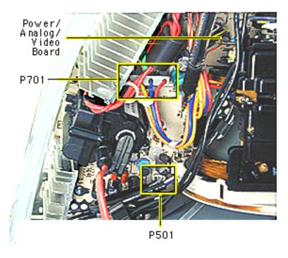
Disconnect P501 and P701 on the power/ analog/video board. The cables are located near the high voltage capacitor.
