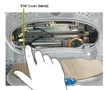
Touch the metal EMI shield inside the recessed latch area before touching any components on the main logic board.
