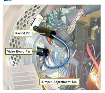
. Connect the jumper adjustment tool (922-4165) to the video board pin. Refer to the "Jumper Adjustment Tool" procedure mentioned earlier in this section.
