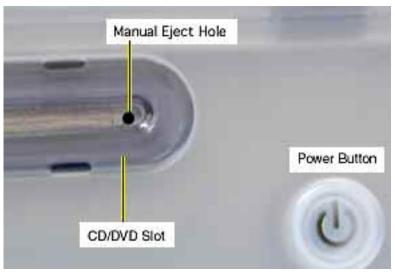
If the CD/DVD discs still won't eject after pressing the manual eject button, remove the bottom housing, and then replace the bottom housing ensuring that the center tab of the bottom housing is properly aligned.
