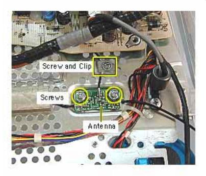
1. Remove the three screws and cable clip on the antenna.
