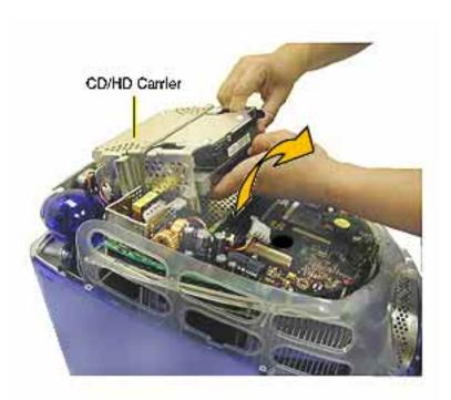
Tilt the CD/HD carrier forward and lift the carrier out of the computer.
