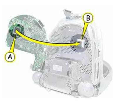
The thermal pad (A) and the divider panel(B) are used on the following logic boards:
