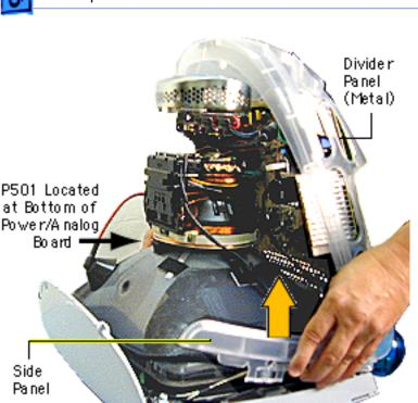
7. Partially lift the side panels (with the power/ analog/video board attached to the divider panel) up and off the inner bezel to gain access to connector P501 located at the bottom of the power/ analog/video board.
