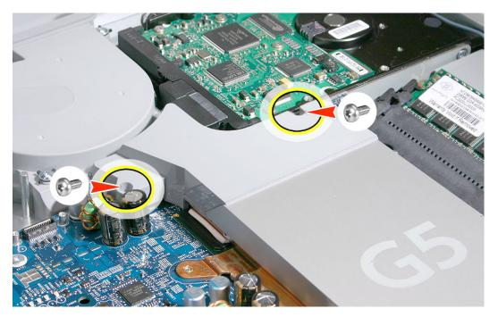
4. Remove the three hard drive screws. Next, lift the hard drive up a bit and disconnect the hard drive data and the hard drive power cables on the left side. Lastly, disconnect the thermal sensor and the inverter cable (located near the copper heatpad).
