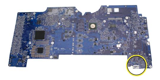
6. Before placing the logic board into the midplane chassis, position the cables out of the way so they don't get stuck under the logic board.
