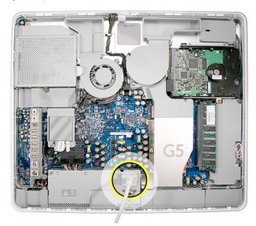
3. Press the power button with your finger or a nylon probe tool. The LEDs will come on indicating the computer status.
