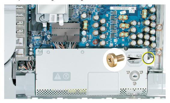
22. Turn the middle case screw counterclockwise about five revolutions. This step prepares the back cover to be installed and secured.
