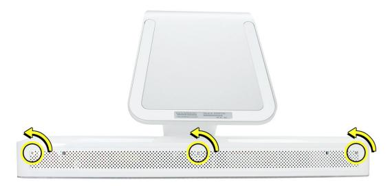
6. Holding the back cover by the metal foot, tilt the cover up and lift it off the computer. Set the back cover aside
