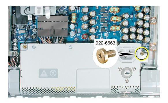
6. Turn the middle case screw counterclockwise about five revolutions. This step prepares the back cover to be installed and secured.
