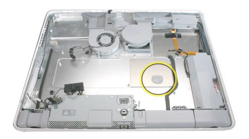
4. Add 1 1/2 to 2 syringes of thermal grease to the U3 chip to ensure sufficient cooling. Spread the paste evenly across the surface of the chip.
