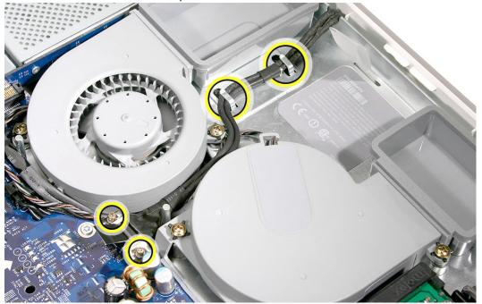
3. Depending on the type of screws present (Torx 8 or Phillips #2), loosen the two fan screws. **Note:** You don't have to remove the screws from the rubber grommets to remove the fan, just loosen the screws.
