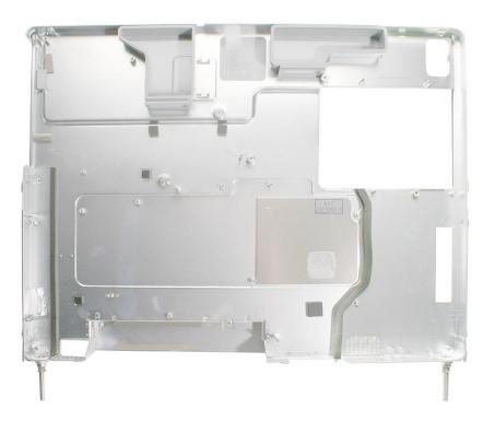
2. On the other side of the chassis, note that the midplane chassis includes the mesh tape that borders the hard drive area.
