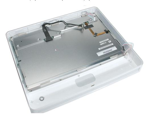
3. Make sure that the black video cable is tucked into the groove on the bezel as shown. Use the screw hole (smaller circle) as a guide for the cable placement.
