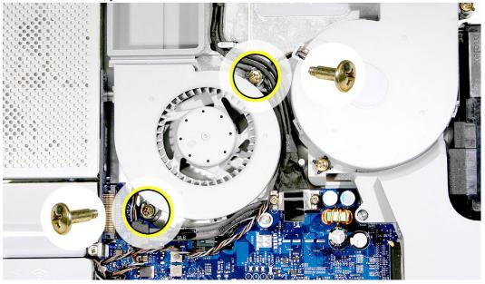
9. Disconnect the fan cable from the connector on the logic board. Pull on the black connector, not on the cable.
