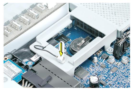
7. With the nylon probe tool, push the battery in the direction of the arrow to free the battery from the metal clip.
