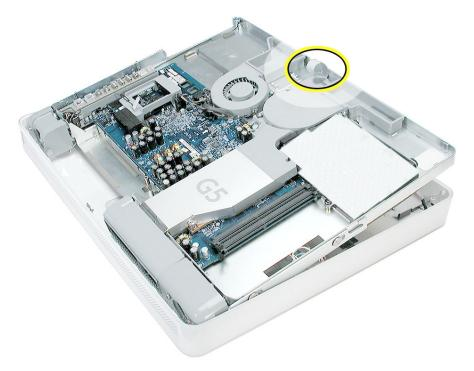
6. As you lower the midplane, pull the inverter cables through the openings on the right side of the midplane.
