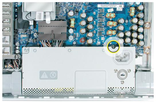
15. To unlatch the power supply, tighten the middle case screw by turning it clockwise five to eight revolutions.
