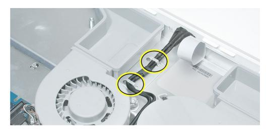
35. Flip the cable back, so it is out of the way for the next step.
