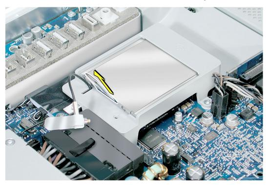
6. Reconnect the antenna cable to the hole on the AirPort card guide.
