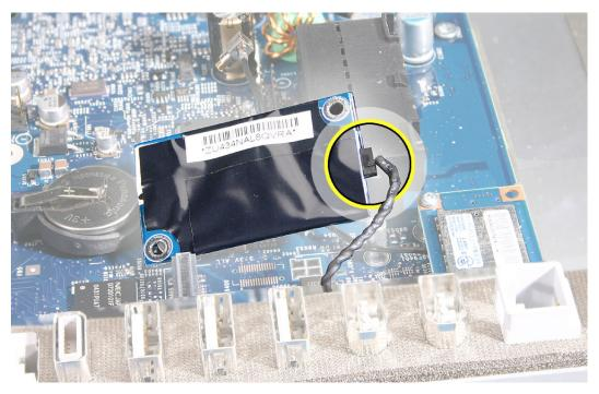
15. Connect the modem to the logic board and replace the two modem screws.
