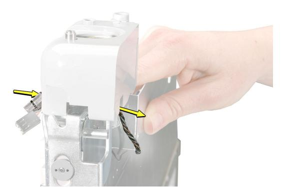
3. Without straining any of the cables, use a flat-blade screwdriver to carefully pry open the cable guides on the underside of the midplane chassis. Release the fan cable from the cable guides.
