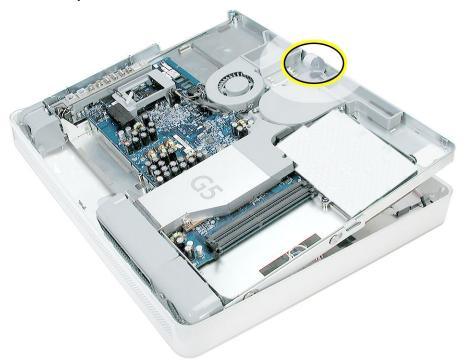
37. Push the inverter cables down through the openings on the midplane assembly. Lift the midplane assembly up and set it aside. **Important:** Return this midplane to Apple in the packaging provided
