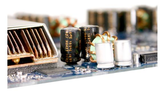
11. If the logic board has bulged or vented capacitors, replace the logic board as well. Refer to the next topic in this section, Special CompTIA Codes, for repair coverage information.
