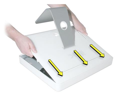
3. Lower and press the cover into place until it fits snugly on the computer.
