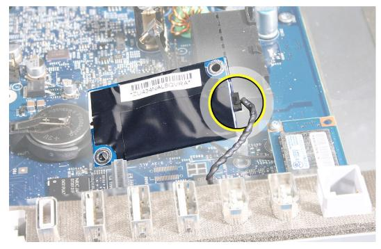
8. Using a T-6 screwdriver, remove the two screws on the Bluetooth board.
