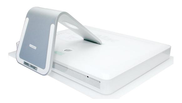
4. Raise the foot and use a Phillips #1 screwdriver to loosen the three screws at the bottom of the computer by turning them completely counterclockwise. These are "captive screws," which means they're not supposed to come all the way out.
