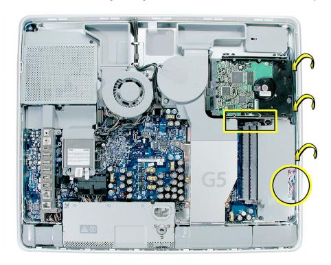
13. Replace the memory module(s) by lining up the notch on the module with the notch on the slot. Press firmly on the memory module until it clicks into place. Use your thumb and index finger to push the module into the slot.
