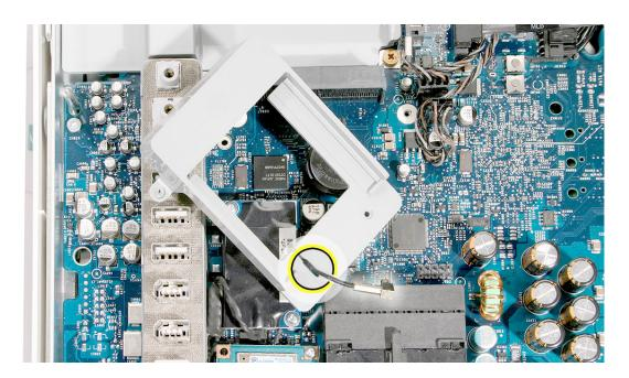
2. Fit the AirPort Card holder onto the logic board. With the AirPort Card holder properly aligned and level, replace the two screws.
