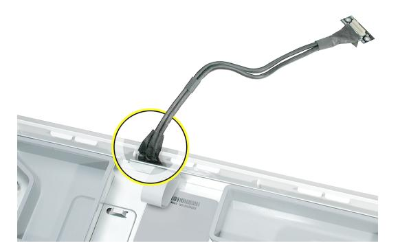
36. Locate the pull tab. Pull the tab up to release the midplane assembly from the display/bezel assembly.
