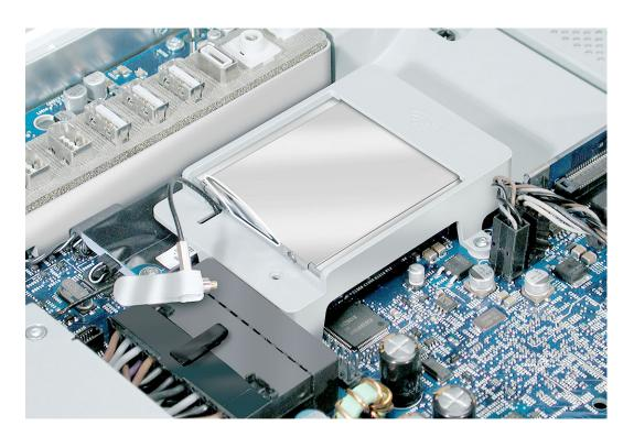
27. Connect the antenna cable to the end of the installed AirPort Extreme card.
