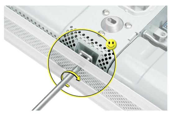
29. Lift up the power supply at the sides approximately five mm or until it touches the middle case screw.
