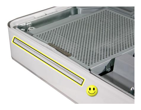
9. Replace the four optical drive screws.
