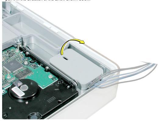
14. Disconnect the two white connectors underneath the cover. Pull on the connectors, not on the cables. Free the cables from the clips inside the cover. Set the inverter and cable cover aside.
