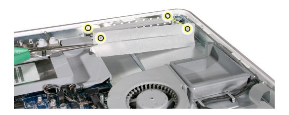
4. Tuck the mircofoam into place before installing the optical drive.
