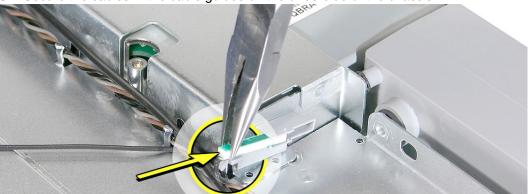
**Replacement Note:** If necessary, use a flat-blade screwdriver to press the cable guides closed over the cables.
