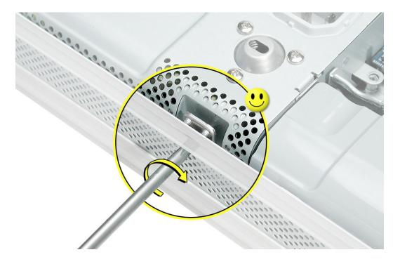
16. Remove the six screws (four identical, short, brass-colored screws in the channel along the top, and two screws on the left side of the board).
