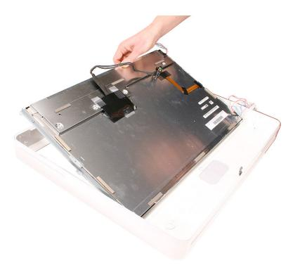
4. Holding the top and bottom edges of the panel, lift it out of the bezel.
