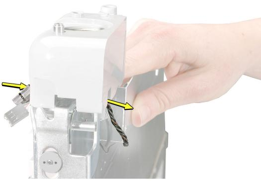
4. Route the microphone cable connector through the midplane chassis opening.
