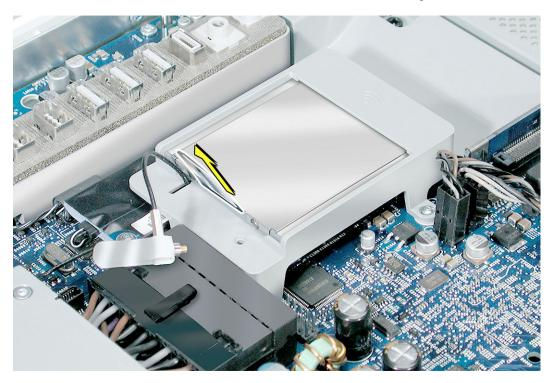
24. Reconnect the antenna cable to the hole on the AirPort card guide.
