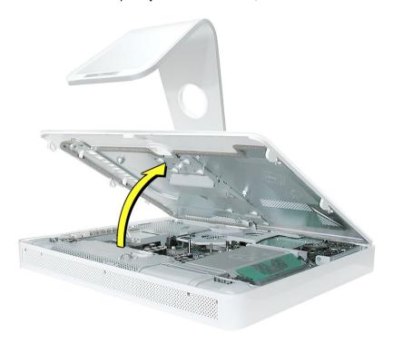
6. To protect the computer from electrostatic discharge, ground yourself by touching a metal surface inside the computer. Warning: Always discharge static electricity before you touch any parts or install any components inside the computer. Don't walk around the room in socks or bare feet, for example, until after you've finished these steps.
