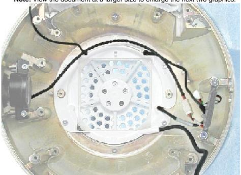
2. There are five screws on the neck cap, however; only the three silver screws need to be removed. The remaining two black screws keep the neck attached to the base.
