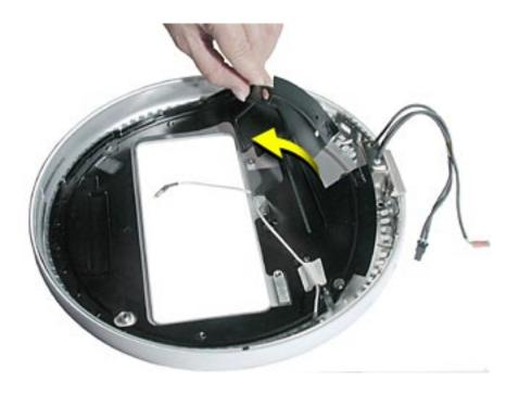
Remove two screws and lift the AC line filter from the bottom housing. Note: The AC line port cover plug may fall out of the bottom housing when you remove the AC line filter. Place the plug back into the bottom housing before reinstalling the AC line filter.
