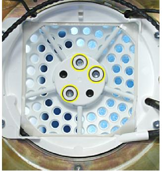
3. Llift the neck cap off the cables. Tthe two remaining black screws hold the neck to the base. Note the orientation for neck reassembly.
