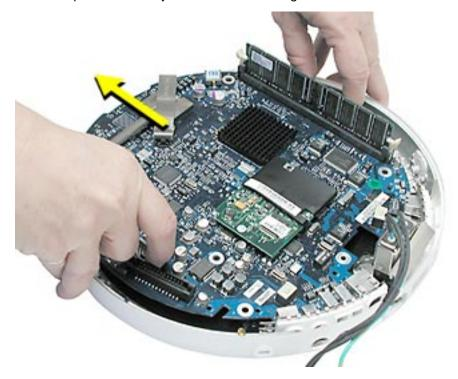
Remove the I/O port covers from the logic board.
