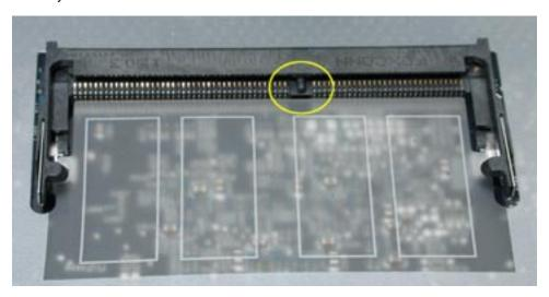
2. **Important:** Do not push the clips (circled below) when inserting memory. They are used to remove memory from the slot, not to insert memory. These clips are fragile and can break.
