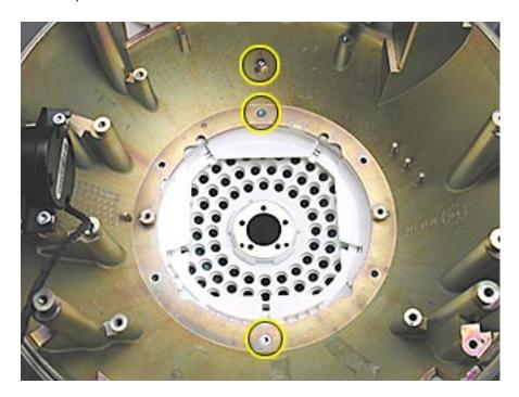
2. Separate and lift the Faraday cage away from the outer housing. Be careful not to scratch the white plastic housing. Important: The Faraday cage is very heavy and has sharp edges; handle with care.
