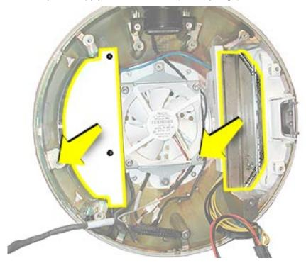
4. **Replacement Note:** When replacing the metal plate (see picture above) that sits on top of the power supply , make certain that the two shorter screws are inserted into the screw holes near the optical door. If the longer screws are inserted by mistake, the screws will scratch the top housing (circled below).
