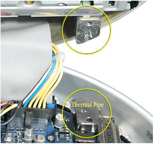
2 Squeeze a drop of thermal paste onto the middle of the thermal pipe surface as shown below.
