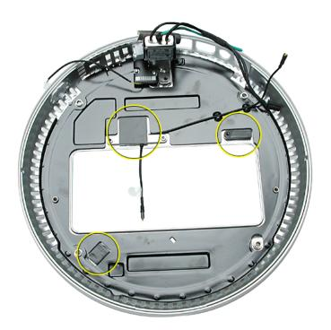
Warning: Whenever the logic board is removed, you must install new thermal pads to three surfaces (shown above). Failure to apply these pads could cause the computer to overheat and possibly damage the internal components. Note: An exception would be if you are simply testing the logic board and only detach it for a few minutes.
