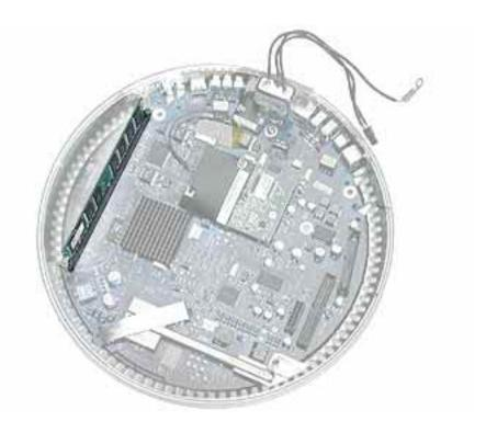
Note: The factory-installed memory slot is identified as Slot J13 by Apple Hardware Test and Apple System Profiler.
