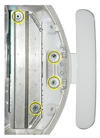
3. Remove the power supply from the chassis (Faraday cage).
