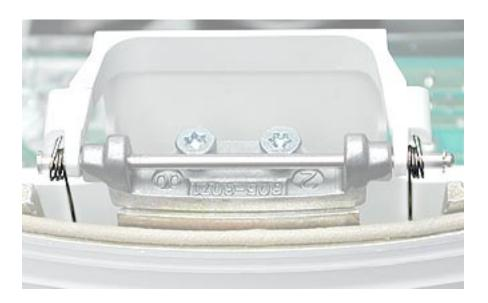
4. Remove the door hinge screws.
