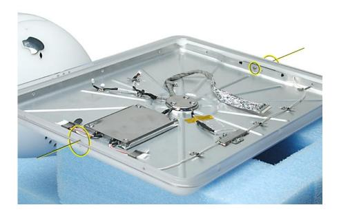
2. Remove the two internal antenna screws on the sides (shown by the circles) and the two 5mm nuts connecting the wireless antenna to the panel shield.
