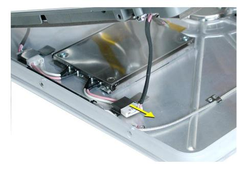
5. Raise the display to disconnect disconnect the circled items: the antenna, the inverter cable, the microphone, and the power on LED. Then, peel the tape away from the video connector and open the clip to release the video cable (see next page for a close up of the clip). Note: View this page at a larger size to enlarge the graphic.
