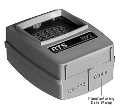
If you suspect the light meter is giving false readings, verify the readings with a known-good light meter or photometer. Also check the age of the R77 light meter by its four-digit manufacturing date stamp (such as 0398 for March 1998).
