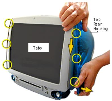
5. Position the computer right side up. Push down and pull out on the rear housing to unhook the rear housing tabs that connect to the inner bezel.
