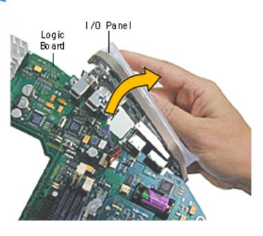
Rotate the logic board right side up again.
