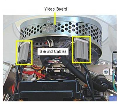
2. With the power off, remove the left ground cable from the video board.
