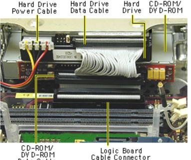
**Note:** Remove SDRAM to make cable removal easier.
