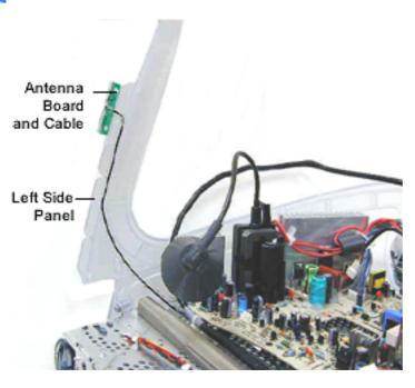
Carefully remove the antenna from the left side panel. Refer to the next page for a close up of the antenna in the left side panel.
