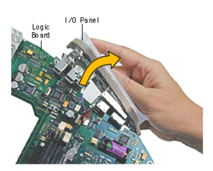
Rotate the logic board face up again and carefully slide the I/O panel off the logic board.
