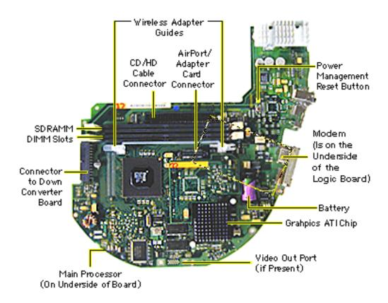
iMac 350 MHz Logic Board Diagram
