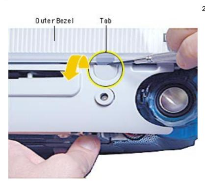
2. After removing the tabs, remove the screws located under the tabs.
