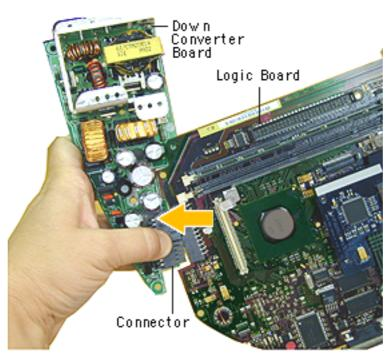
6. Holding onto the boards, press down on the black connector and separate the down converter board from the logic board.
