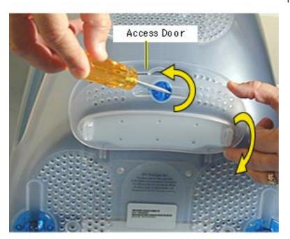
With a flatblade screwdriver or coin, turn the colored latch to open the access door.
