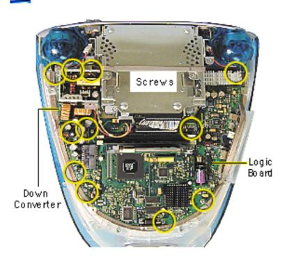
Remove the six screws on the logic board and five screws on the down converter board.
