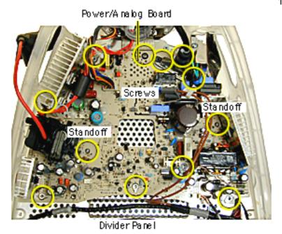
15. Remove the ten screws and pinch the two standoffs with a needlenose pliers to lift the power/analog board off the divider panel.
