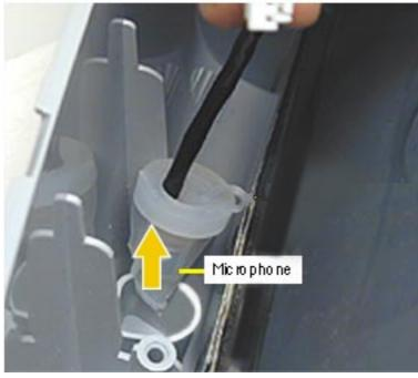
3. Pull the microphone from the inner bezel.
