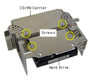
Note: The hard drive carrier shown was removed from the computer. However, you can easily remove the hard drive while the carrier is still screwed down to the chassis. Continue with the procedure.
