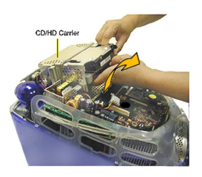
Tilt the CD/HD carrier forward and lift the carrier out of the computer.
