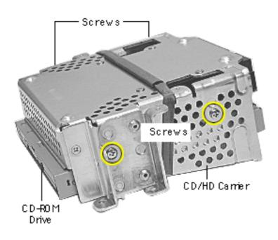
Using a Phillips screwdriver, remove the CD/HD carrier mounting screws (two on each side).
