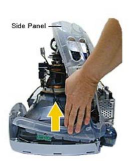
5. Pull the panels out to the sides a bit, and then lift the side panels up and off the computer.
