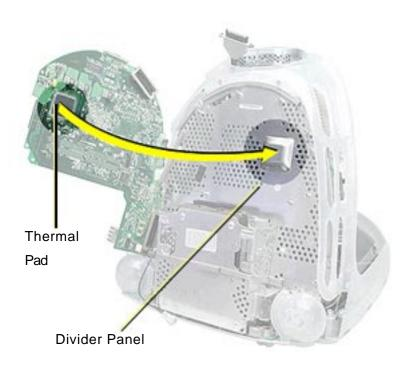
Install the logic board back on to the divider panel.
