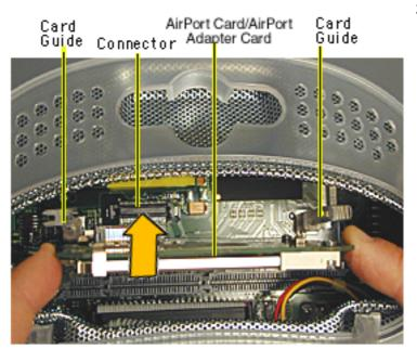
Remove the AirPort Card by lifting the card straight up and out of the card guides and connector.
