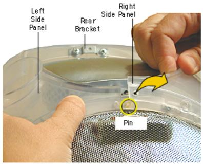
4. At the top rear of the side panels, pull each side panel off the plastic pin.
