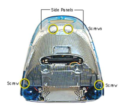
On the rear of the side panels, remove four screws. These screws connect the side panels to the divider panel (the metal chassis).
