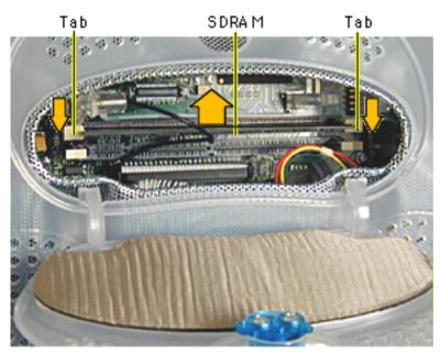
4. Push the ejector tabs on the slots outward and down so they are in the open position.
