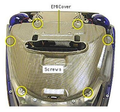
1. Remove the six screws on the EMI cover.
