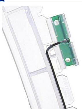
Important: Note how the antenna wire is routed through the side panel before removing. A close-up view of the right panel antenna is shown here.
