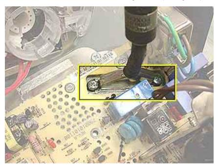
Figure 3 RGB Cable Connection
