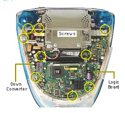
3. Remove the six screws on the logic board and five screws on the down converter board.
