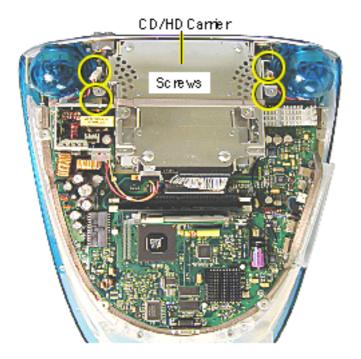
Remove the four screws connecting the CD/HD drive carrier to the metal chassis (also known as the divider panel).
