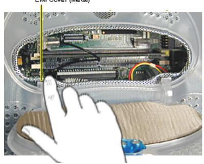
Touch the EMI cover that is visible inside the recessed latch area before touching any components on the main logic board. This protects the computer from damage caused by electostatic discharge
