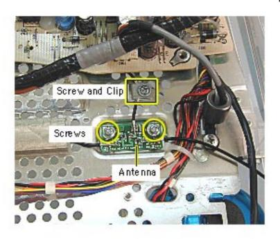
Remove the three screws and cable clip on the antenna.
