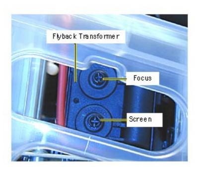
Adjust the focus control on the flyback transformer until the focus test pattern reaches the best frontof-screen performance.
