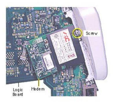
3. Turn the logic board over and remove the modem screw.
