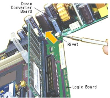
Using a flatblade screwdriver, pry the rivet off the logic board.
