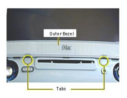
With a jeweler's screwdriver, carefully remove the two tabs on the front outer bezel. Refer to the next graphic for a close-up of the tab removal.
