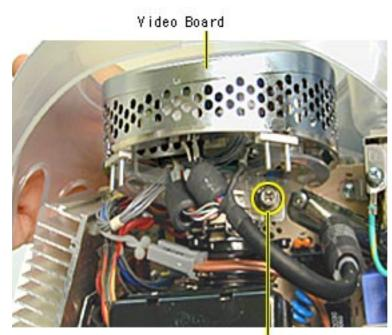
12. Loosen the CRT neck clamp screw.
