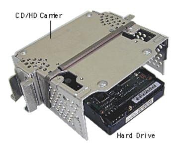
3. Slide the hard drive out of the CD/HD carrier.
