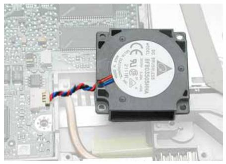
Install the replacement fan, and reassemble and test the computer.
