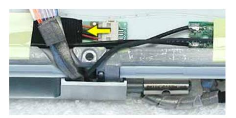
6. Remove the reed switch cable assembly.
