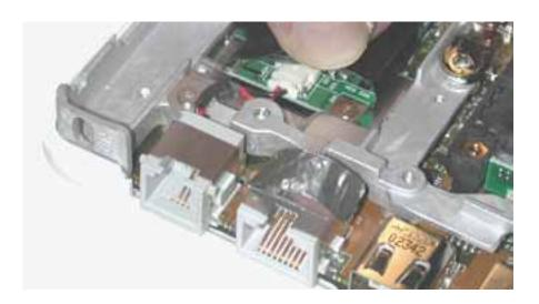
4. Slide the modem port forward and off of the logic board.
