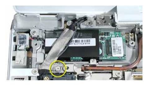
2. **Important:** Do not strain or remove the LVDS cable.
