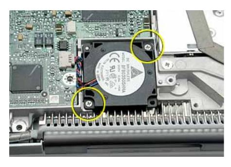
2. Lift the fan from the computer, and use a black stick to disconnect the connector from the logic board.
