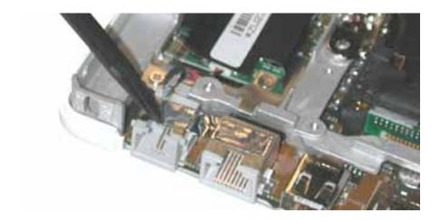
3. Lift up the modem sleeve and disconnect the RJ11 modem cable from the modem board.
