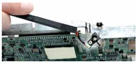
3. Remove the two screws holding the vent cover to the heat spreader.
