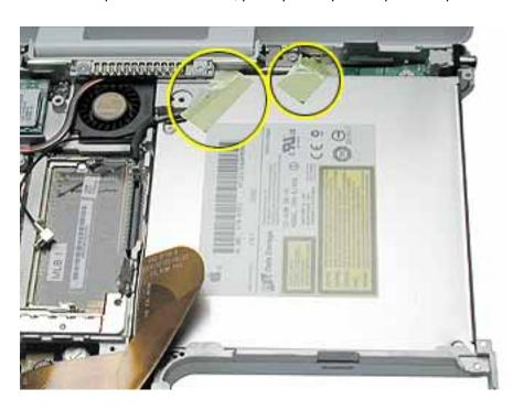
2. Remove the two screws from the tabs at the upper left area of the optical drive.
