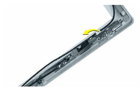
7. At the bottom of the bezel, remove the tape from the inverter board and note the routing of the two soldered cables on the left side of the antenna board.
