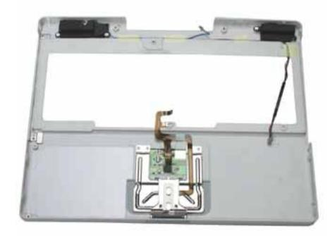
20. Install the replacement top case, and reassemble and test the computer.
