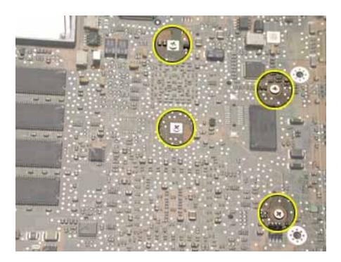
5. Turn over the computer frame, and remove the remaining screw at the heat spreader plate.
