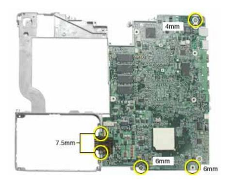
8. Lifting the logic board at the back ports, tilt up the logic board to remove it from the frame.
