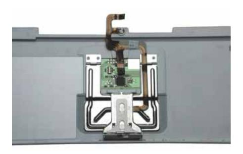
3. Use a black stick to lift up the ends of the connector that holds the trackpad cable to the board.
