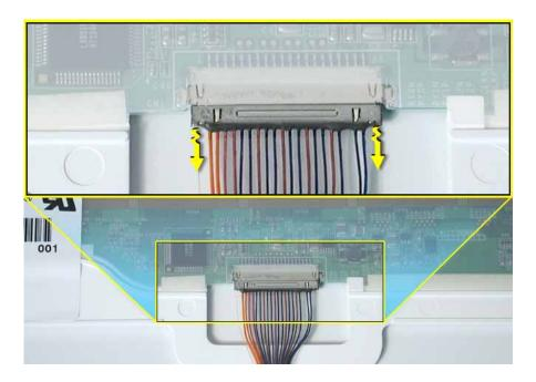
12. At the other end of the LCD cable, remove the tape from the bottom edge of the LCD panel.
