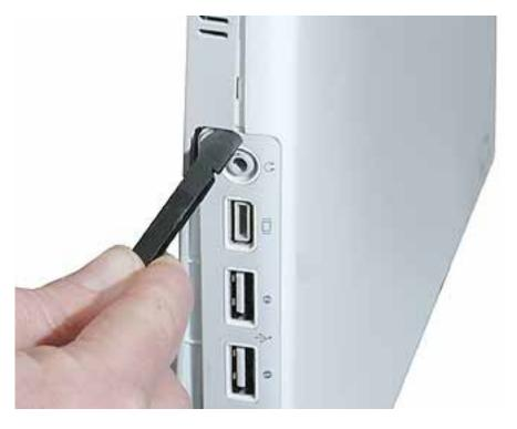
11. While continuing to loosen the top case, use caution around the battery bay. If necessary, flex the inner frame to release that corner of the top case.
