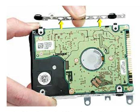
7. Install the replacement hard drive, and reassemble and test the computer.
