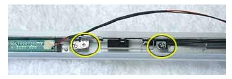
9. Tilt up the antenna receptor to remove it from the left side of the bezel assembly.
