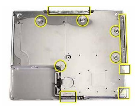
4. Peel up the tape at the computer latch. If the tape tears, replace it with new aluminum tape.
