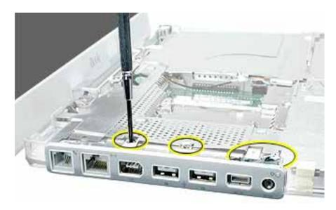
2. Tilt down the I/O bezel and remove it from the computer frame.
