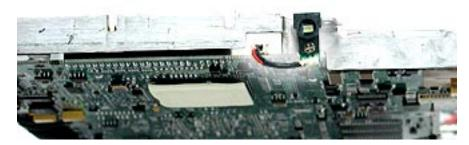
2. Using a black stick, disconnect the sleep light board connector from the logic board.
