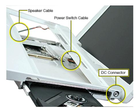
10. With the top case loosened, note how the speaker cable is routed.
