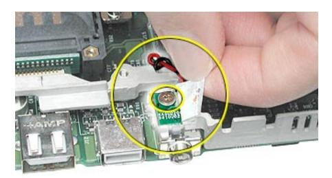
4. Remove the two screws holding the vent cover to the heat spreader.
