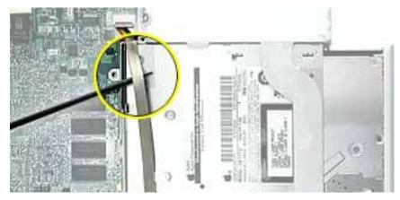
2. Remove the single screw from the DC board.
