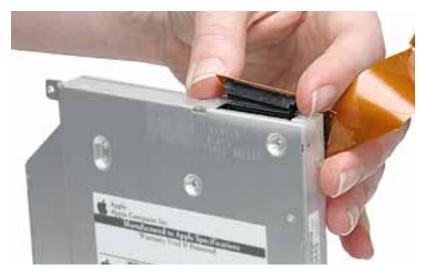
9. Remove the drive door and install it on the replacement optical drive, as described in the next section.
