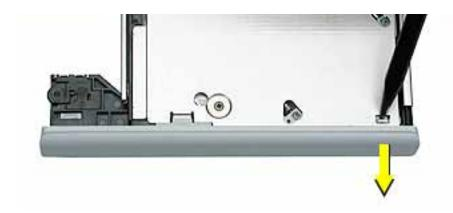
3. Press the wider tab, and pull the door off of the drive.
