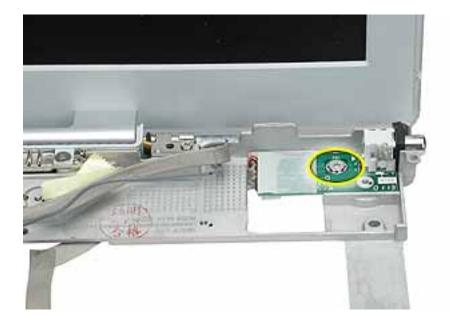
3. Tilt up the computer and note the routing of the flat power cable across the underside of the inner frame.
