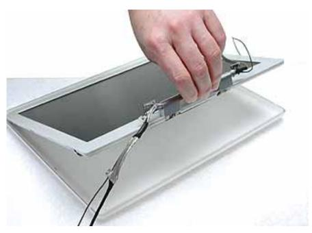
4. Place the display assembly face down on a soft cloth.
