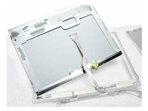
14. Disconnect the inverter cable from the inverter board at CN2 and remove the LCD panel.
