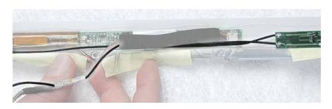
8. On the left side of the bezel, remove the two 3-mm long Phillips screws at the antenna receptor.
