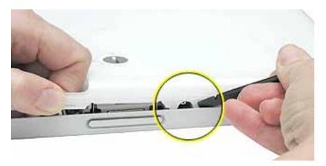
11. Carefully work the black stick around the corners of the bottom case.
