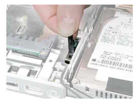
3. Peel the tape off of the optical drive, and disconnect the flat backlight cable from the logic board.
