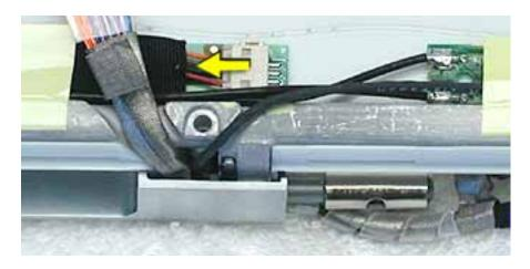
6. Remove the reed switch cable assembly.
