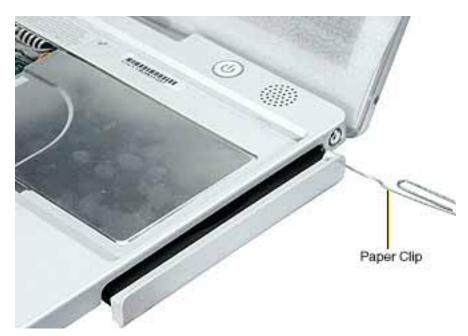
7. Warning: Avoid pressure on the optical drive rail. The space between the drive rail and the rightmost screw (shown below) is very tight. When removing that screw, putting pressure on the drive rail can damage the drive. If necessary, refer to the Optical Drive procedure, "Transferring the Drive Door" to remove the drive door first; then slide in the optical drive tray and remove the screw.
