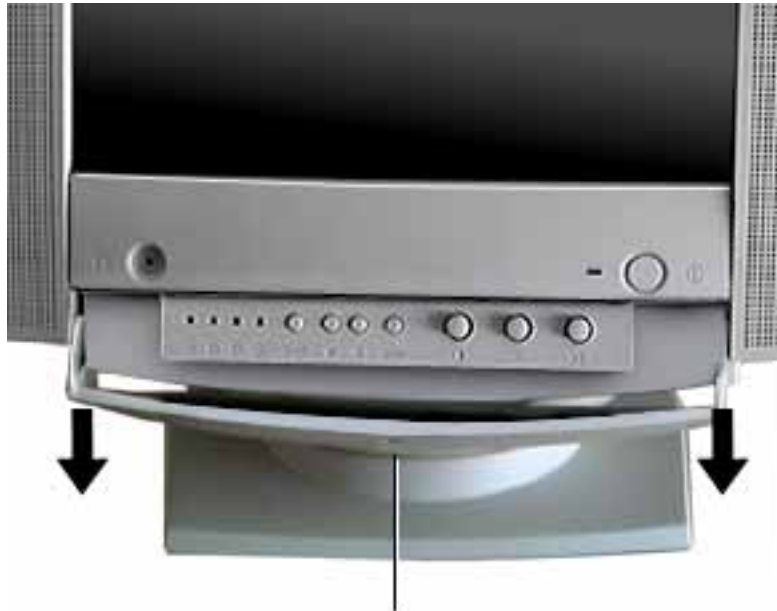
Control Panel Door
