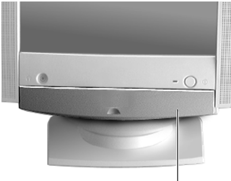
Control Panel Door
