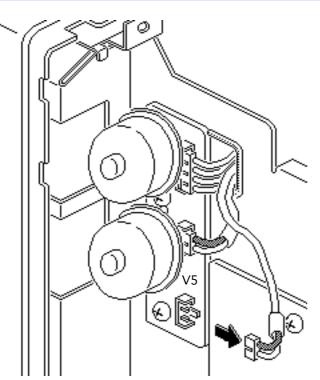
4 Disconnect the cable at location V-5 from the contrast control board.
