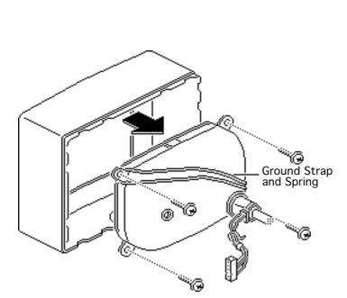
3 Remove the four CRT mounting screws and lift the CRT out of the bezel.
