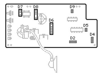
**Note:** Connectors D2, D4, D5, and D9 fit tightly and are difficult to reach, so pull the main board away from the chassis before you try to remove these connectors.
