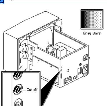
If you adjust the cutoff control (RV506) up (clockwise) too far, the monitor may shut down. If this happens, turn off the monitor and turn down the cutoff control fully counterclockwise. Wait 30 seconds, turn on the monitor, and resume the adjustment.
