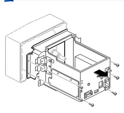
2 Remove the six chassis mounting screws and pull the chassis off the bezel.
