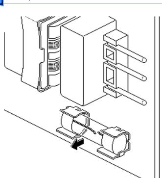
If the wire inside the fuse is broken, replace the fuse (250 V, 2 A).
