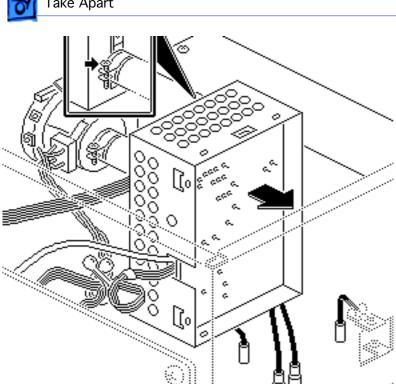
Caution: Twisting, bending, or applying force to video board C could damage the neck of the CRT. Be sure to pull video board C straight off the neck of the CRT.
