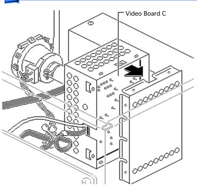
Replacement Note: Video board C is in a metal box. When replacing a defective board, retain the back cover of the metal box and send the rest of the module, including cables, back to Apple.
