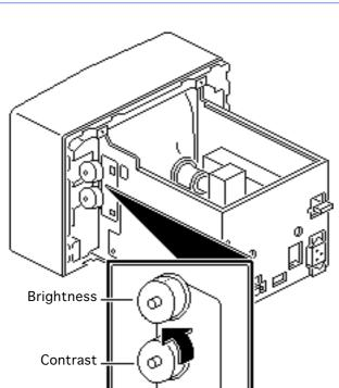
Set the contrast knob to maximum and the brightness knob to the center (detent) position.
