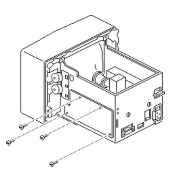
1 Remove the four screws that fasten the main board to the chassis.
