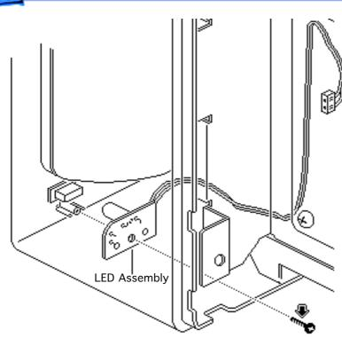
3 Remove the LED mounting screw and lift the LED assembly free.
