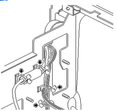
2 Remove the cables from the four plastic clamps.
