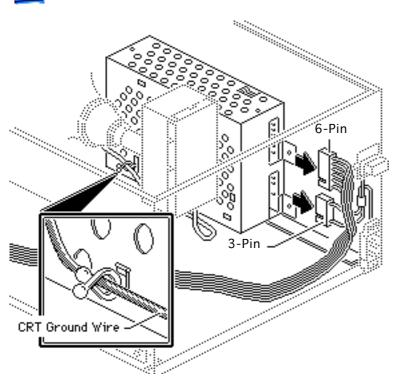
**Note:** To disconnect the 3pin connector from the power supply, you may need to remove tie-wraps from the power supply cable. Then lift the chassis and reach beneath the power supply.
