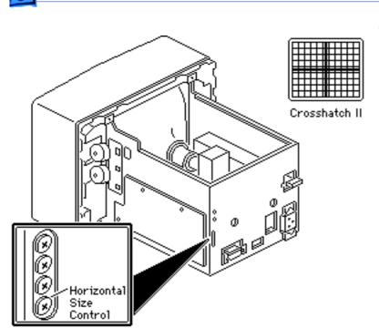
2 Using a plastic screwdriver, adjust the horizontal size control until the raster is 8.4 inches (213.5 mm) wide.
