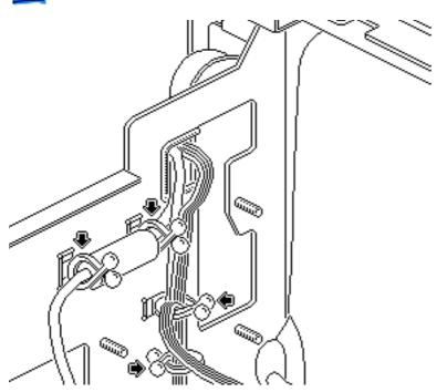
1 Remove the wires from the four cable clamps.
