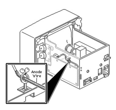
2 Remove the anode wire from the cable clamp.
