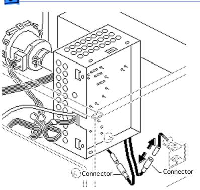
5 Disconnect the two black cables from the bottom of video board C at their midpoint connectors.
