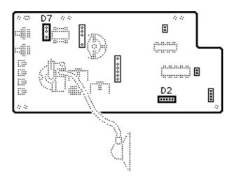
Disconnect connectors D2 and D7 from the logic board.
