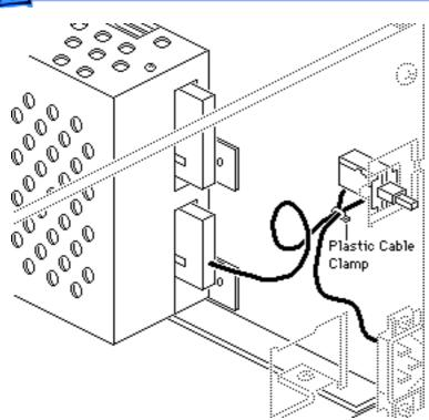
Remove the two wires from the plastic cable clamp and desolder the wires from the switch.
