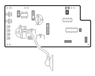
Disconnect the two-pin connector from location D9 on the main board.
