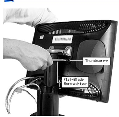
7 Using a flat-blade screwdriver, loosen but do not remove the two thumbscrews and thin plastic washers at the rear of the display.
