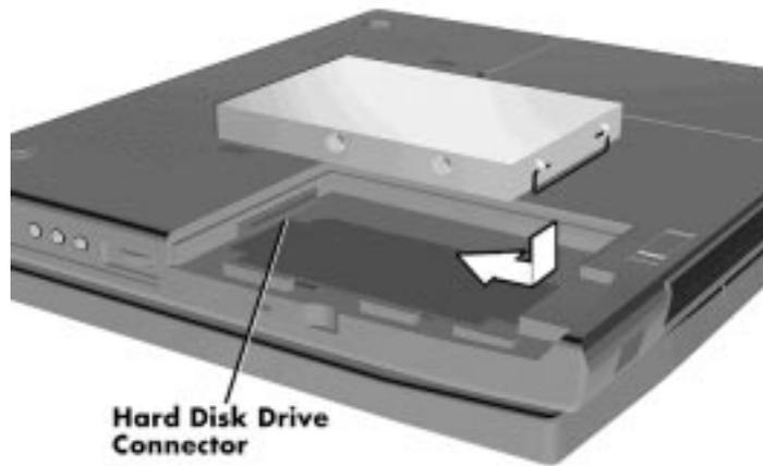
*Inserting the hard disk drive*
