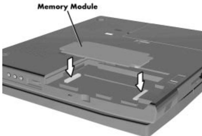
*Inserting the memory module*
