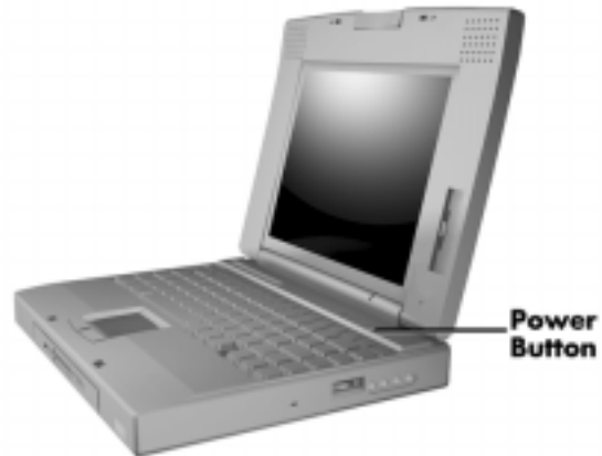
Powering on the system
