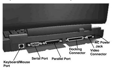
**Keyboard and Mouse Port** — Use the standard PS/2 port to connect an external PS/2 mouse or an external PS/2 keyboard. If you want to connect both, use the optional NEC Versa Y Adapter. (See the online *NEC Versa 2000 Options Catalog.*)
