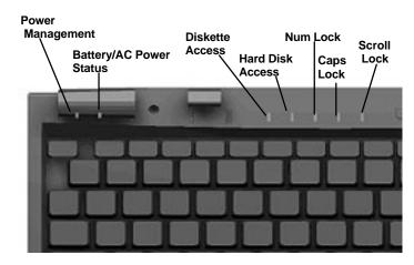
**Power Management** — Green when on; no color when off. Blinking green when the system is in Suspend mode.
