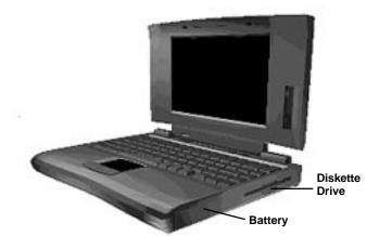
**Diskette Drive** — You can save your files to diskette and install software from diskette using the diskette drive, called drive A.
