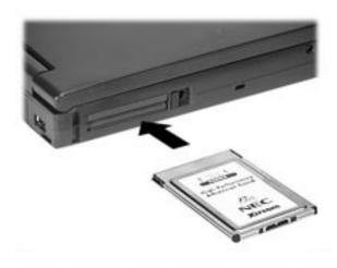
Inserting a PC card
