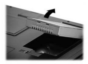
Removing the battery pack
