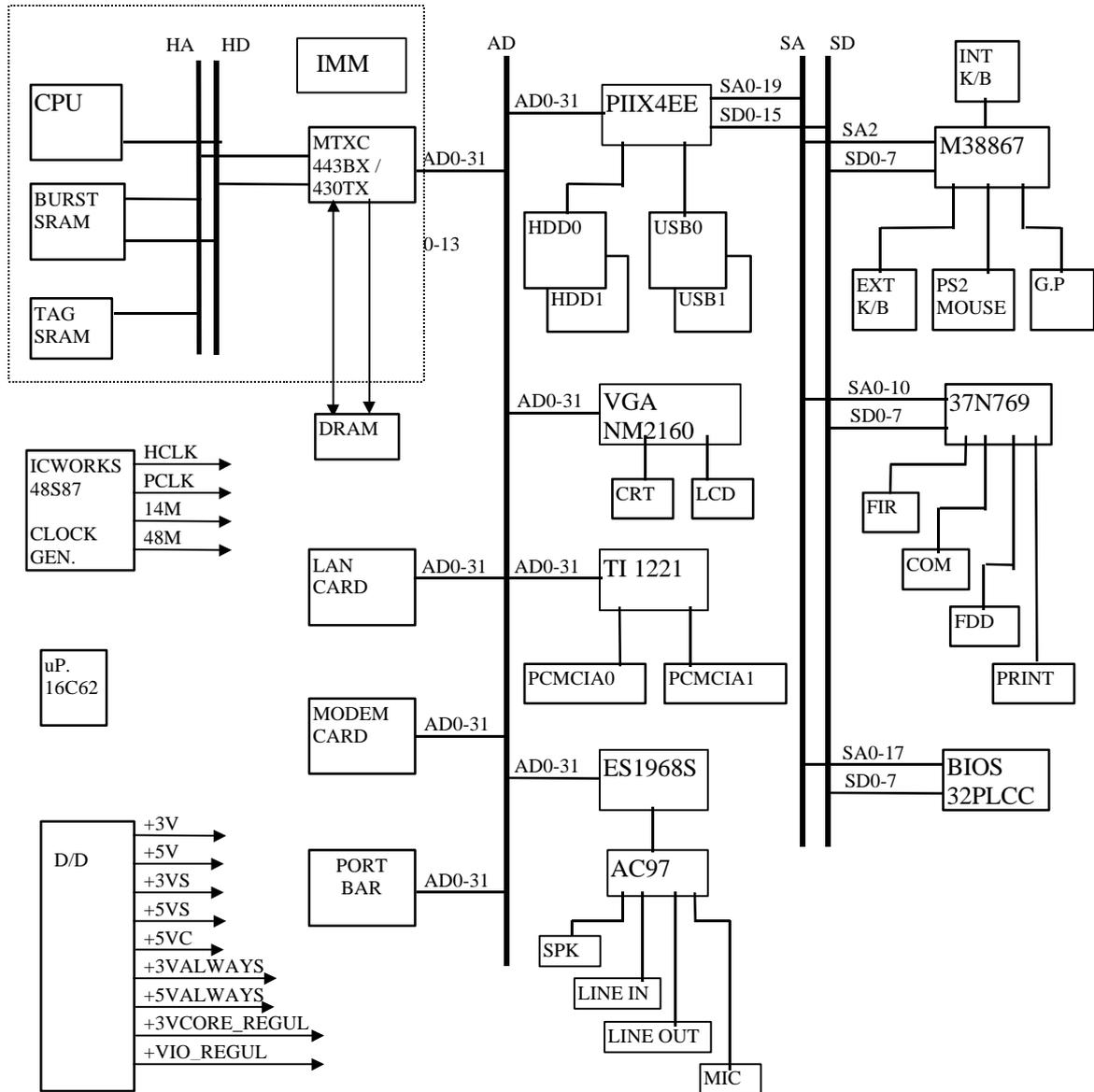
**Note:** The Video, PCMCIA, and Sound subsystem are PCI-bus design. All of the core commands are synchronized by PCI clock to improve performance.
