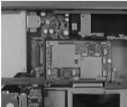
7. To insert the CPU module again, fit in the CPU module into the connectors and make sure it fits snugly. Then, secure the screws again.
