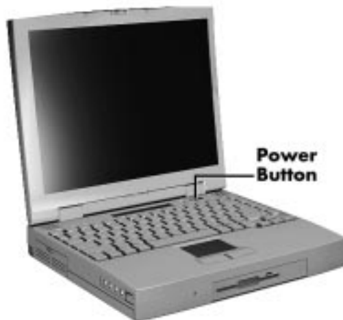
Figure 2-2 Powering on the System
