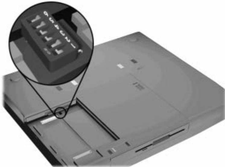
Figure 2-12 Locating the Switch Settings
