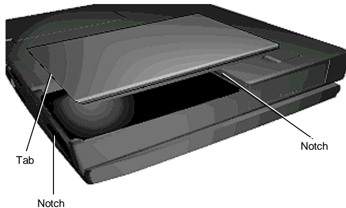
Figure Section 2-11 Battery Bay Cover Replacement
