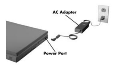
Figure 2-1 Connecting the AC Adapter
