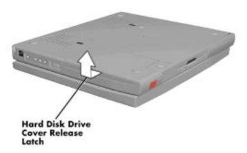
Figure 4-1 Removing the Drive Bay Cover
