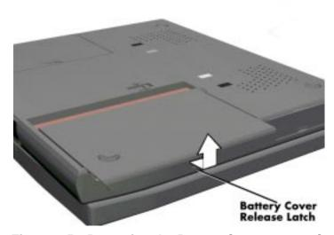
Figure 4-5 Removing the Battery Compartment Cover
