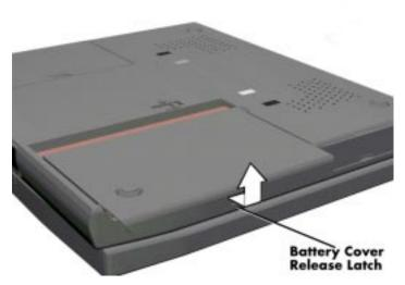
Figure 2-5 Removing the Cover
