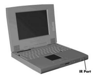
Figure 1-8 Front IR Assembly Location
