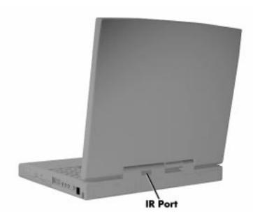
Figure 1-9 Rear IR Assembly Location
