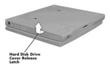
Figure 4-1 Removing the Drive Bay Cover
