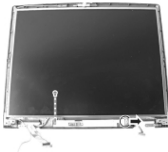
Figure 2-20 Remove the Inverter Board
