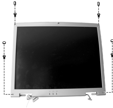
Figure 2-18 Remove LCD frame
