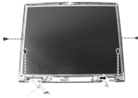
Figure 2-19 Remove LCD panel
