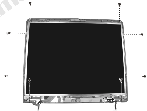
Figure 2-21 Remove the eight screws and disconnect the cable
