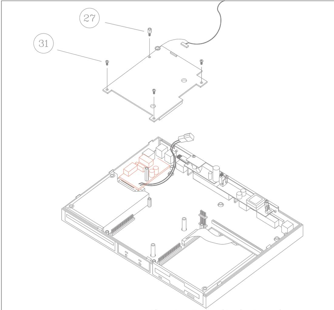
Figure 2-4. Keyboard Section Removal
