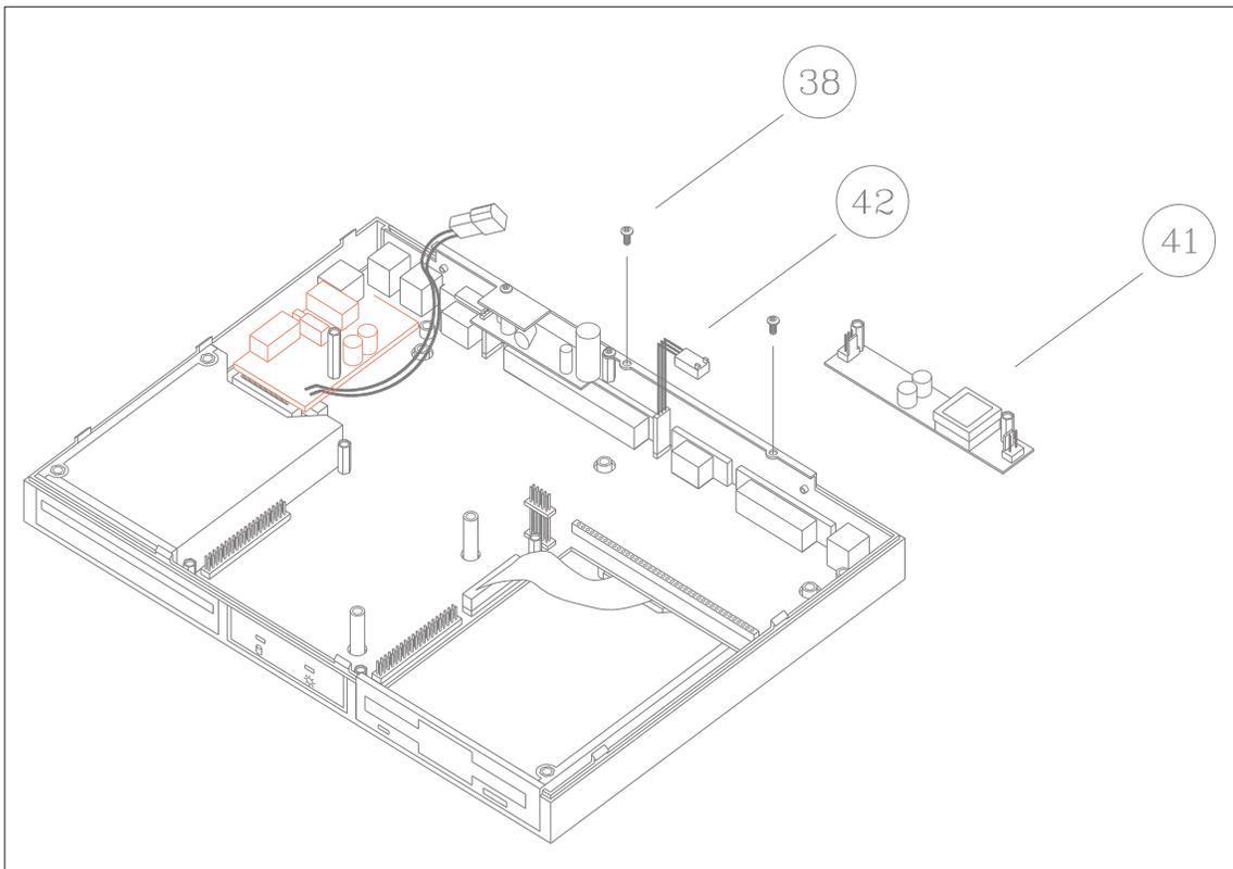
Figure 2-8. DC-AC Inverter Disassembly
