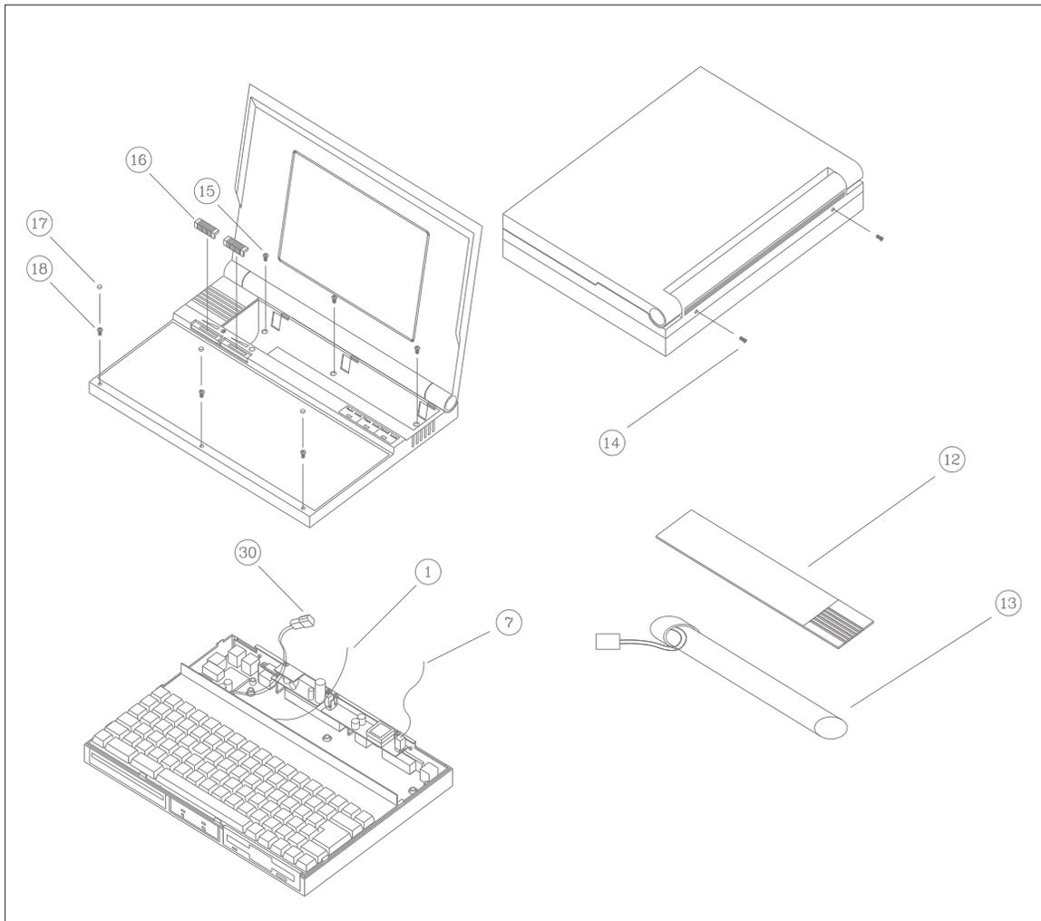
Figure 2-2. LCD Section Removal
