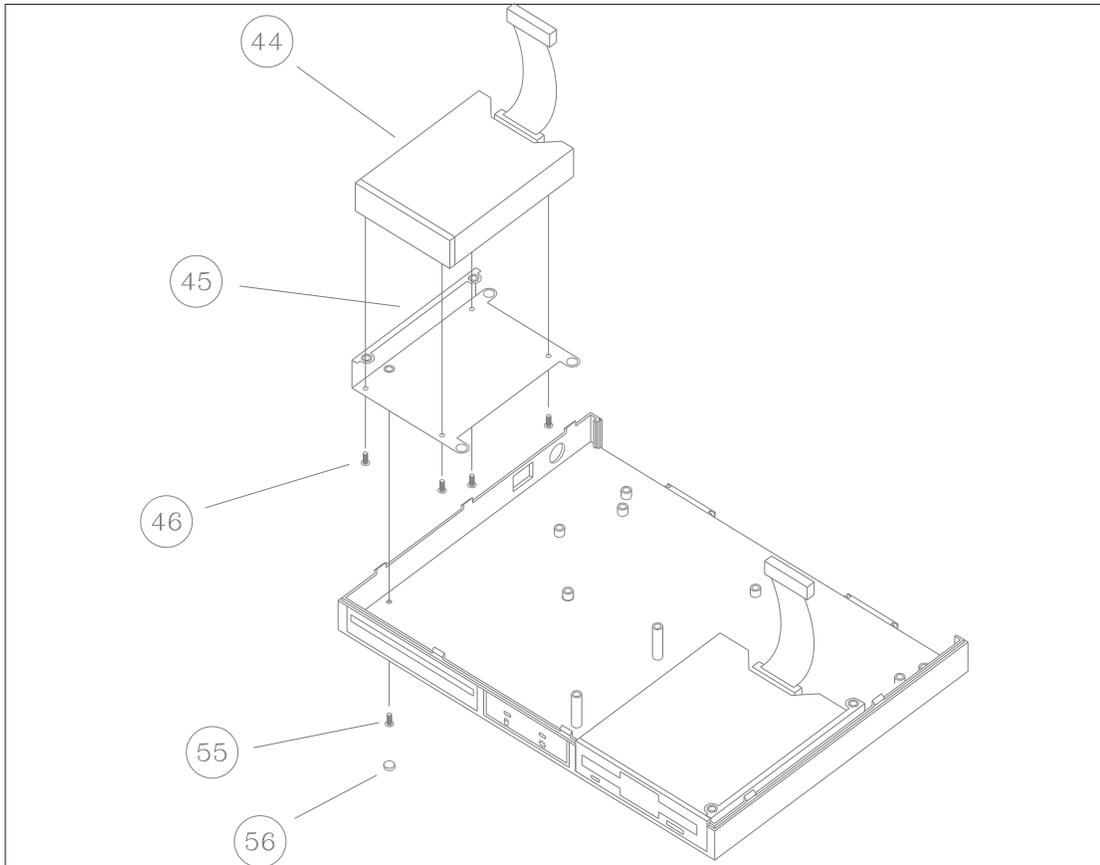
Figure 2-6. Hard Disk Removal
