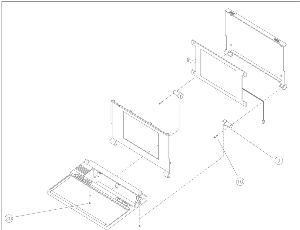
Figure 2-12. Cover Hinge Disassembly
