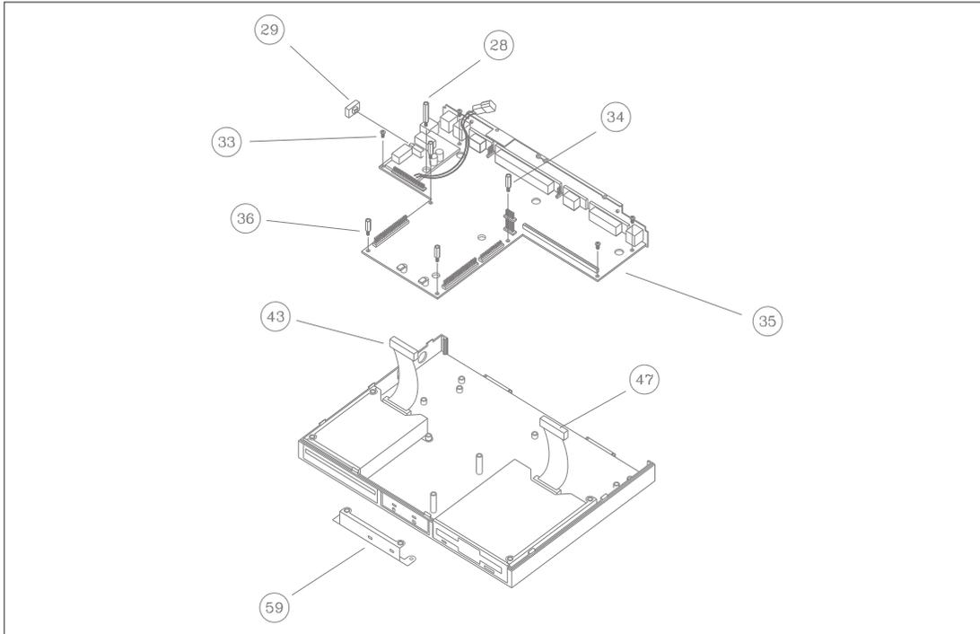
Figure 2-5. System Board Removal
