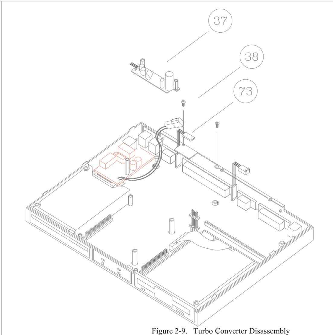
Figure 2-9. Turbo Converter Disassembly
