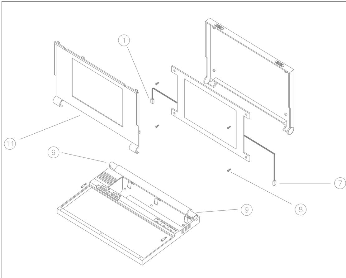
Figure 2-11 LCD Panel Disassembly
