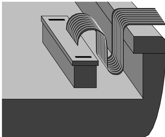
Figure 25 - Proper Keyboard Flex Cable Position
