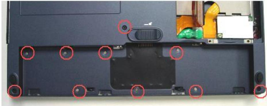
Figure 5-14 Removing the eleven screws of bottom case
