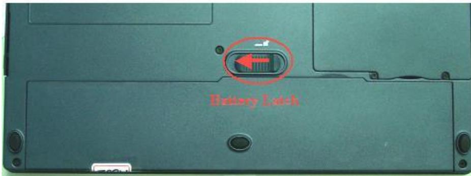
**Figure 5-2 Removing the battery pack**
