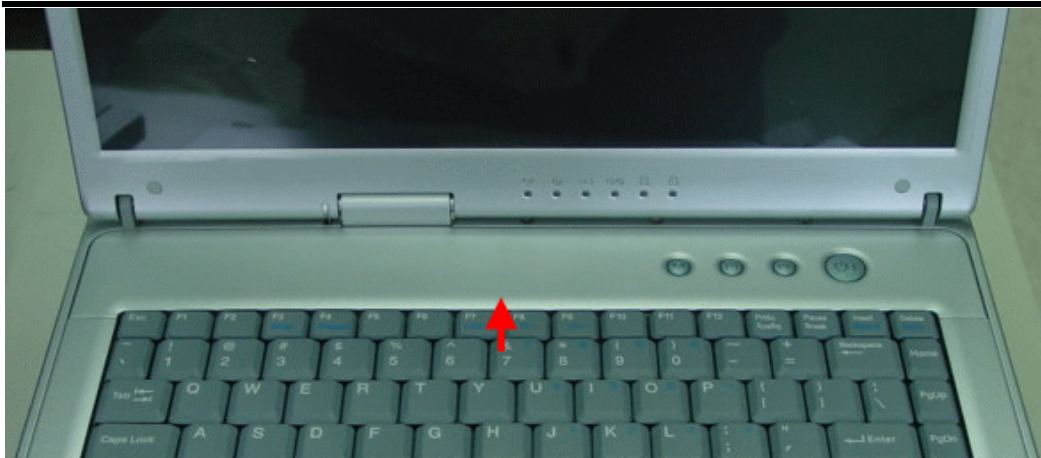
Figure 2-2 Remove keyboard Cover
