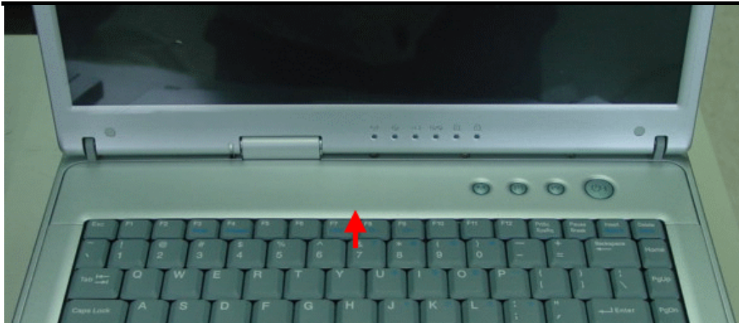
Figure 5-2 Remove keyboard Cover
