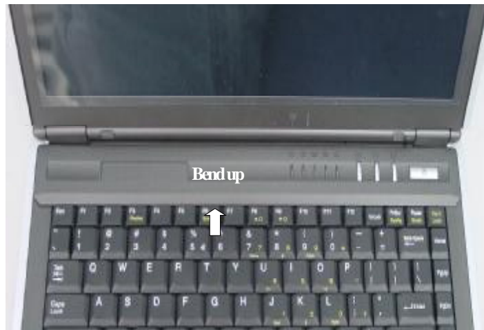
Figure 5-3 Remove Keyboard Cover
