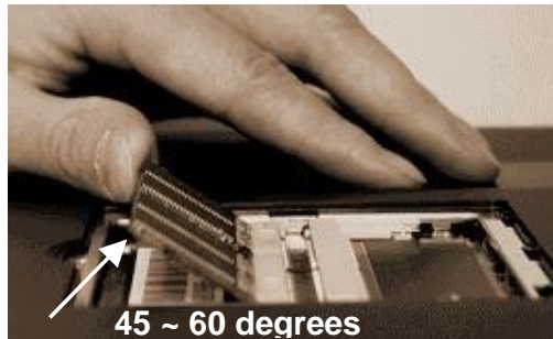
Figure 2-8 Insert Memory Module
