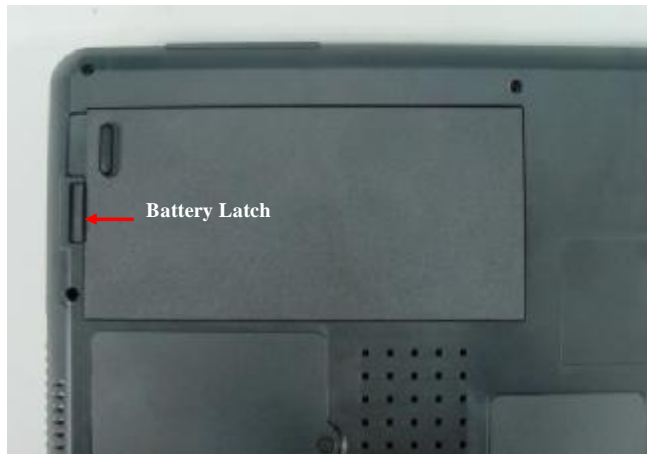
Figure 5-2 Remove Battery Pack
