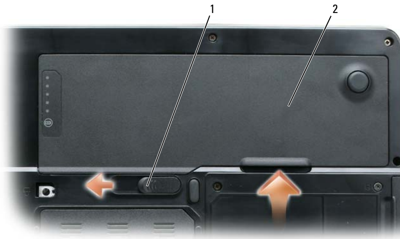
1 battery-bay latch release 2 battery
