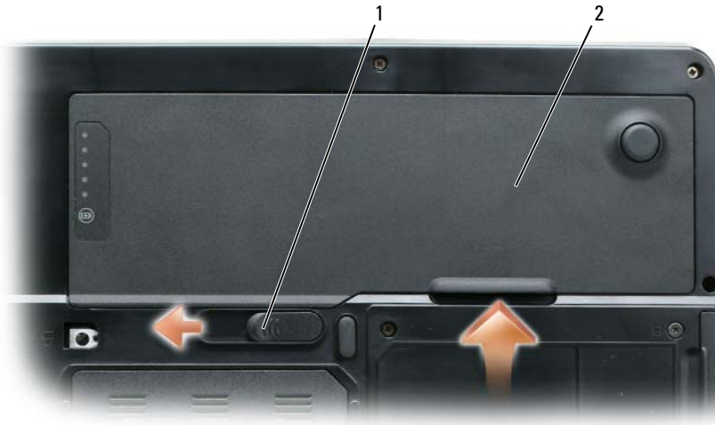
1 battery-bay latch release 2 battery
