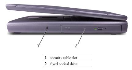
**SECURITY CABLE SLOT** — Lets you attach a commercially available antitheft device to the computer. For more information, see the instructions included with the device.
