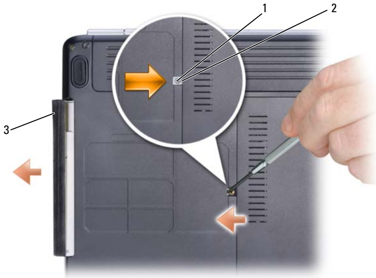
1 locking screw 2 notch 3 optical drive
